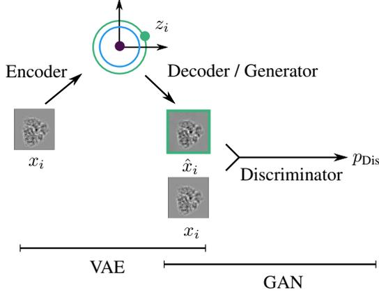
Figure 2. VAE-GAN architecture, illustrated with the simulated images. The encoder encodes the image  $x_i$  into a latent variable  $z_i$ , that is decoded into a reconstructed image  $\hat{x}_i$  by the decoder. The discriminator estimates the probability that  $x_i, \hat{x}_i$  are real images.
