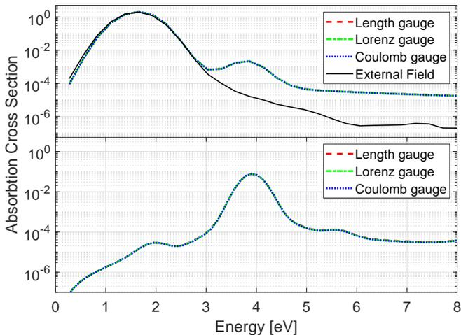
FIG. 5: ACS of 12C for a sine squared pulse (top) and impulse (bottom) as a function of energy for the length (red), Lorenz (green), and Coulomb (blue) gauges.
