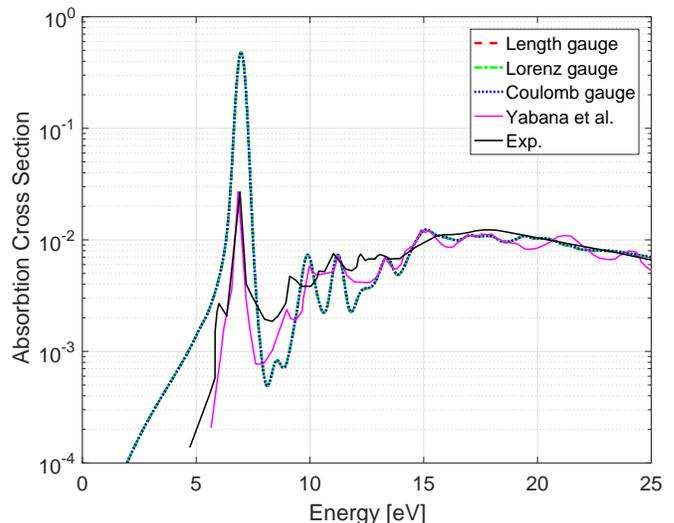
FIG. 3: ACS of benzene for an impulse excitation as a function of energy for the length (red), Lorenz (green), and Coulomb (blue) gauges. Real-time results of Yabana *et al.*<sup>33</sup> (purple) and the experimental results of Koch *et al.*<sup>37</sup> (black) are used for comparison.
