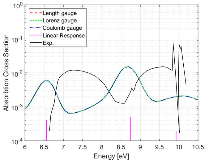
FIG. 1: ACS of water for a boost excitation as a function of energy. Length (red), Lorenz (green), and Coulomb (blue) gauges attained using PARSEC. Comparison is made to the linear response (purple) and experimental (black) results of NWChem<sup>35</sup> and Yoshino *et al.*<sup>36</sup> respectively.
