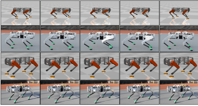
Fig. 6: Comparison between MuJoCo simulation (animated) and experiments. The upper two are for stepping in place, gait4; the lower two are logged for a full step of the ambling gait.
