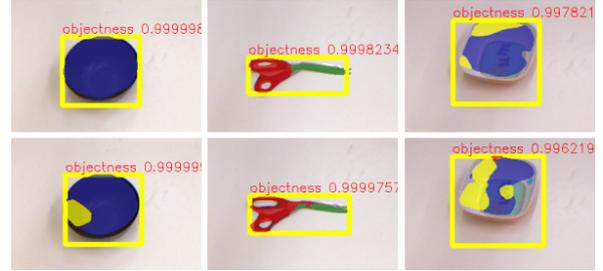
**Figure 7.** Comparison on Cornell dataset. **Top:** detection results of  $AffContext$  method. **Bottom:**  $Obj-wise$  model.
