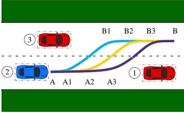
Fig. 1: Sample lane changing sequences that can be chosen by the autonomous vehicle (blue) based on the motion of other non-autonomous vehicles (red) are  $\{(A, A1), (A1, B1), (B1, B)\}$ ,  $\{(A, A2), (A2, B2), (B2, B)\}$  and  $\{(A, A3), (A3, B3), (B3, B)\}$ .
