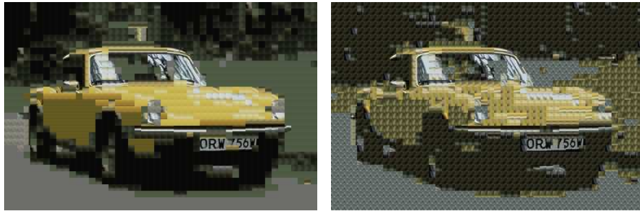
(a) Average distortion minimization, (b) Maximum distortion minimization, compression rate : 5.61%, number of clusters 86 compression rate : 4.82%, number of clusters 74
