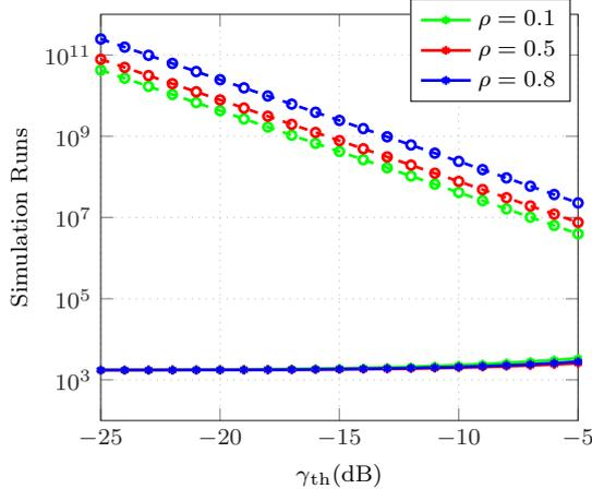
Figure 5: Number of required simulation runs for 5% relative error for 2-branch MRC diversity receivers over correlated Rician fading model with  $E_s/N_0 = 10$  dB. Solid line corresponds to IS and dashed line to MC.
