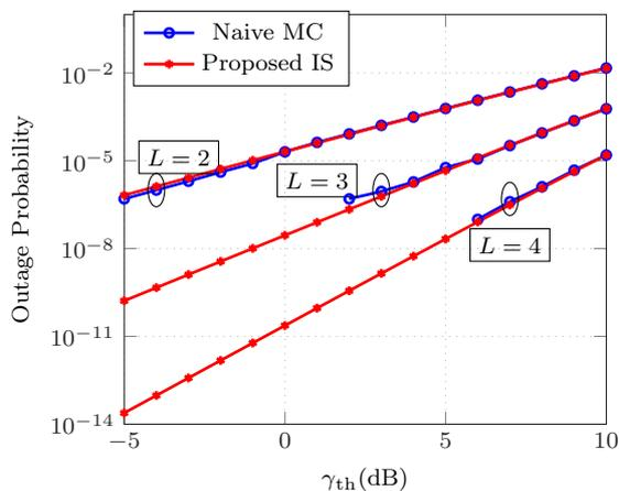
Figure 1: Outage probability of  $L$ -branch MRC diversity receivers over the correlated Nakagami-m fading model with  $E_s/N_0 = 10$  dB. Number of samples  $M = 10^7$  and  $M^* = 10^4$ .
