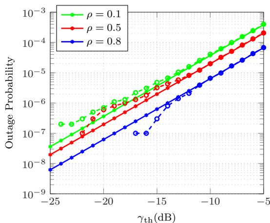
Figure 4: Outage probability of 2-branch MRC diversity receivers over correlated Rician fading model with  $E_s/N_0 = 10$  dB. Solid line corresponds to IS and dashed line to MC. Number of samples  $M = 10^7$  and  $M^* = 10^4$ .
