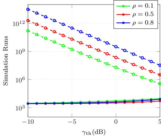
Figure 7: Number of required simulation runs for 5% relative error for 4-branch MRC diversity receivers over the correlated Rician fading model with  $E_s/N_0 = 10$  dB. Solid line corresponds to IS and dashed line to MC.
