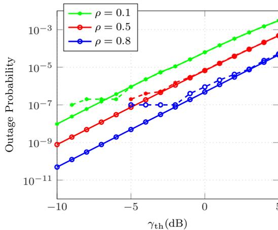
Figure 6: Outage probability of 4-branch MRC diversity receivers over the correlated Rician fading model with  $E_s/N_0 = 10$  dB. Solid line corresponds to IS and dashed line to MC. Number of samples  $M = 10^7$  and  $M^* = 10^4$ .
