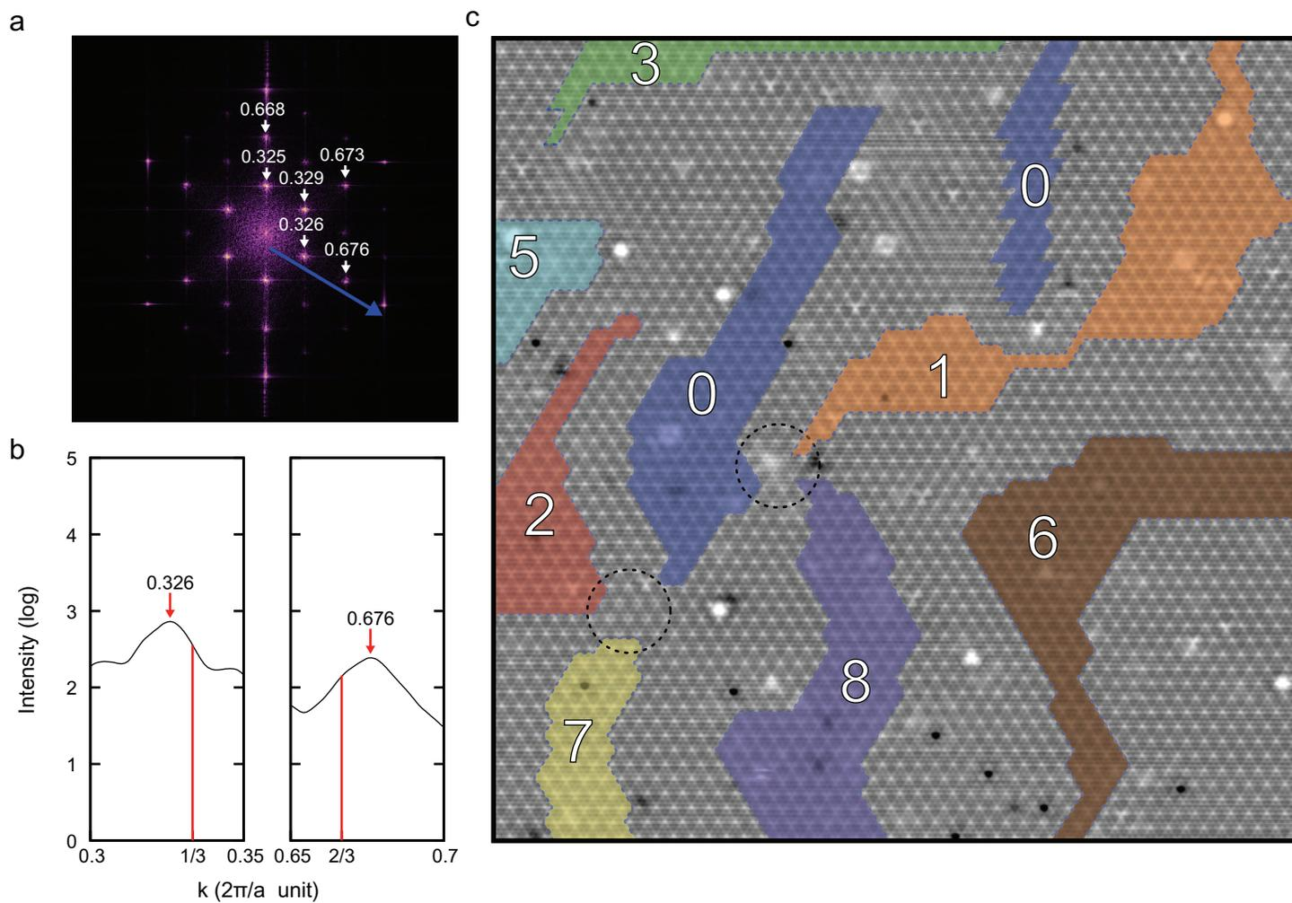
FIGS 7. (a) Fourier transform of the STM image in (c). (b) Peaks in the transformed image near  $1/3$  and  $2/3$  points parallel to the blue arrow in (a). ( $1 \times 1$ ) Bragg peak ( $2\pi/a$ ) is set to 1. (c)  $50 \text{ nm} \times 50 \text{ nm}$  STM topography at a sample bias of 100 mV.
