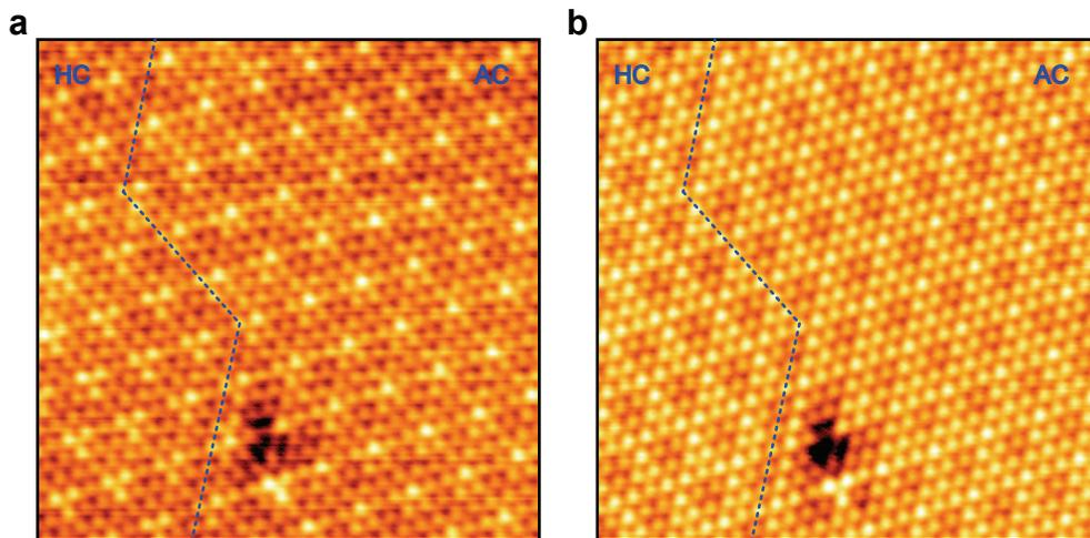
FIGS 1.  $10 \text{ nm} \times 10 \text{ nm}$  STM topography at 100 mV (a) and -100 mV (b). Blue dashed lines indicate the border of two domains. The two distinct domains are clearly observed regardless of bias.
