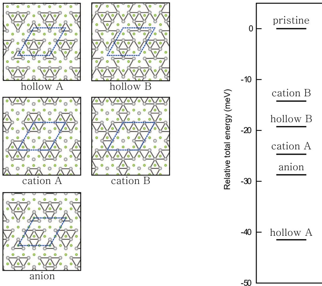
FIGS 2. Atomic structures and relative total energies of five CCDW structures of  $2\text{H-NbSe}_2$ . The CDW structures are categorized according to the center of the structure. Hollow A and anion centered structures correspond to HC and AC structures of the main text, respectively. The total energy of the pristine structure is set to zero. The energetics between HC and AC structure is not significantly altered even with the consideration of magnetic orders.
