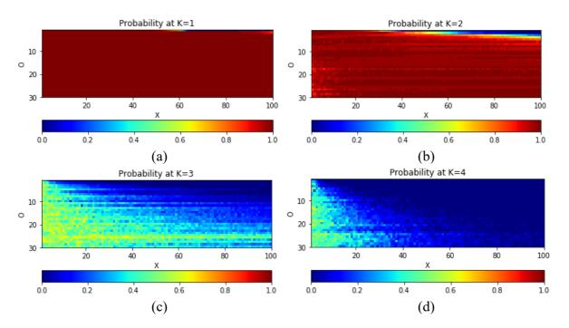
Figure 5: Probability of generating antifragile networks depending on X and O for ordered, critical, chaotic RBNs with N = 100, T = 200, p = 0.5. 50 different networks were used. 10 different initial states were randomly chosen for each network. (a) K = 1. (b) K = 2. (c) K = 3. (d) K = 4.
