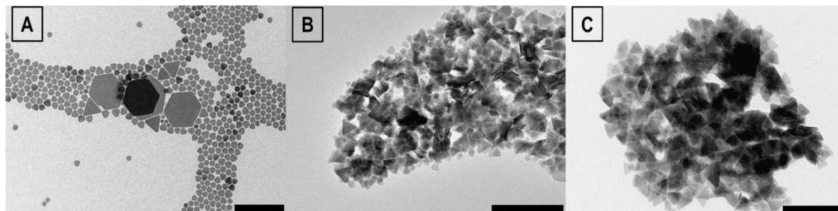
**Figure 2.** TEM images of CuS NCs after 5 min of synthesis by 120°C with Cu:S ratios 0.4:1 (A), 0.2:1 (B) and 0.1:1 (C). Scale bar 200 nm.
