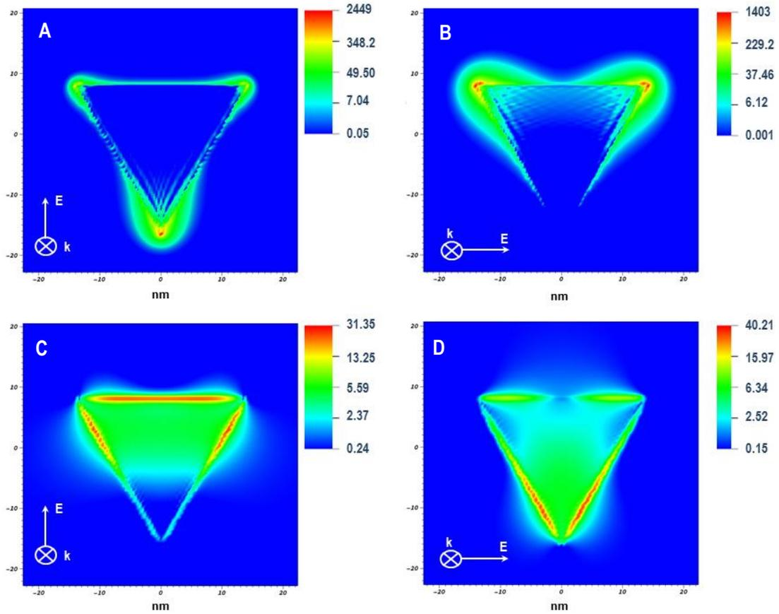
**Figure 8.** Visualization of the near-field intensity ( $|E|^2/|E_0|^2$ ) in triangular CuS nanoprisms. The orientation of  $k$ - and  $E$ -vectors is denoted in the images. (A,B) In-plane intensity distribution at 1650 nm (dipolar LSPR mode). (C,D) In-plane intensity distribution at 1020 nm (quadrupolar LSPR mode). Because of the very high spatial field concentration at 1650 nm, a logarithmic color scaling has been applied.
