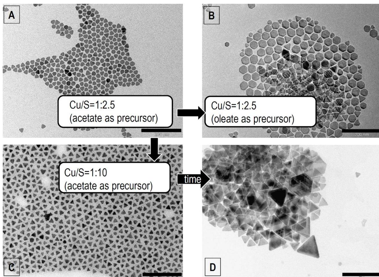
**Figure 5.** Shape changes of  $\text{Cu}_x\text{S}$  NCs during hot-injection synthesis in OAm. (A,B,C) TEM images of samples after 1 min synthesis; (D) after 5 minutes. (A,B) Cu:S ratio 0.4:1, (C) 0.1:1. Preparation of faceted triangles (picture C) with an average side length of 20 nm ( $\sigma=19\%$ ). The size increased with time to  $\sim 50$  nm (D). Scale bars 200 nm.
