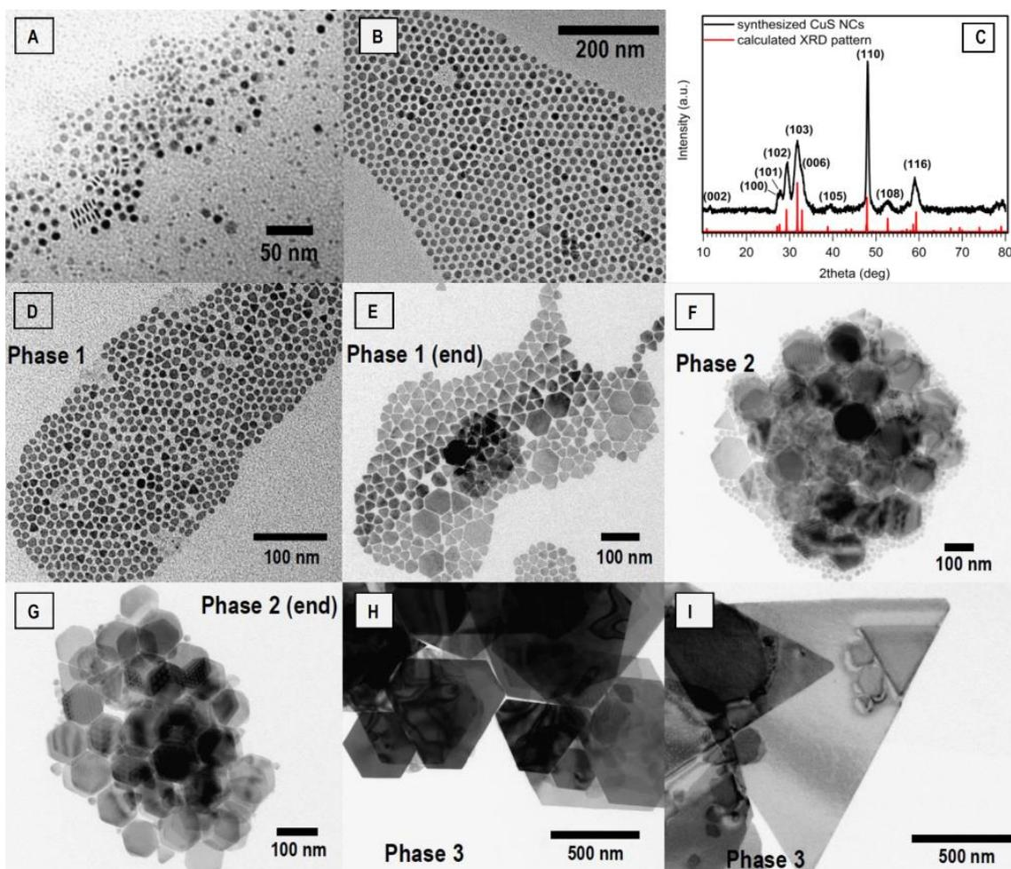
**Figure 1.** Temporal evolution of the  $\text{Cu}_x\text{S}$  2D system under different Cu:S precursor ratios: (A,B) 0.8:1 (1 min, 60 min); (C) XRD pattern of  $\text{Cu}_x\text{S}$  NCs. Reference: calculated profile based on the crystal structure for covellite from Ref. [43]; (D,E,F,G) 0.4:1 (1 min, 30 min, 60 min, 120 min). Reaction temperature 120 °C; (H,I) growth at elevated temperature with precursor addition (160° C for 60 min and 150 ° C for 16 h DPE:OLAM 1:1 vv).
