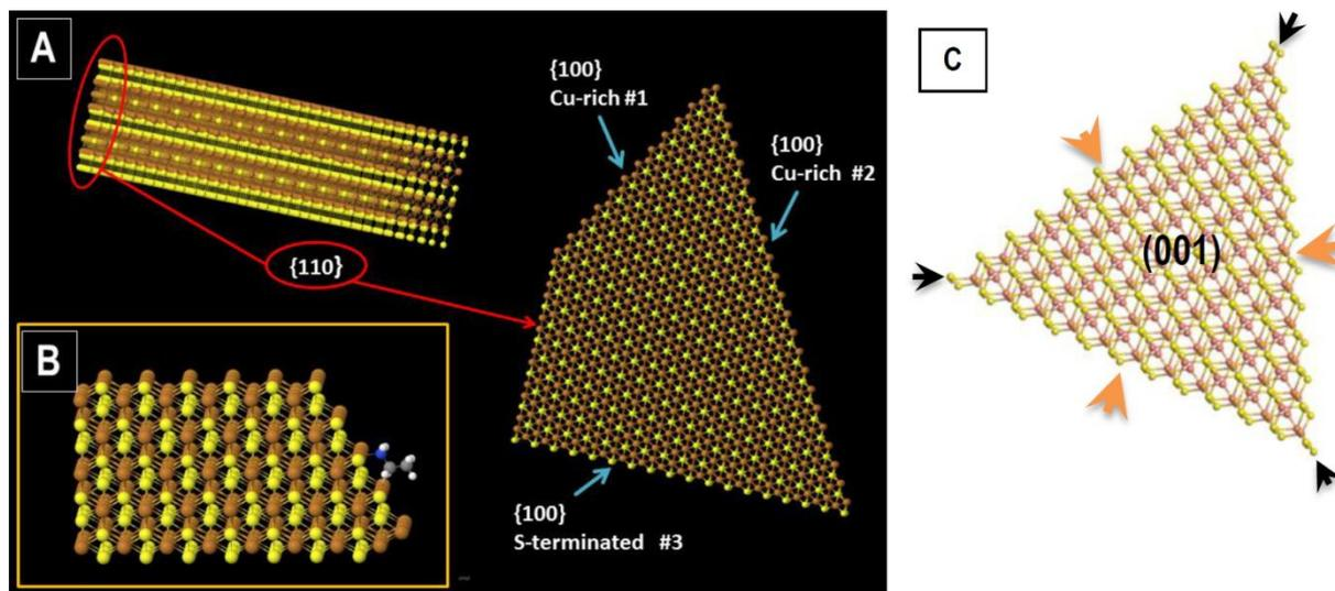
**Figure 4.** Scaled-down atomic models for CuS NCs terminated with different facets: (A) Faceting of the CuS NC according to the simulated surfaces (Table 1); (B) Exemplarily shown amine group adsorbed at {100} facet (#2) (simulation); (C) triangular CuS NC terminated at edges with sulfur atoms, vertex and central positions are denoted by arrows. The lateral crystal plane corresponds to the (001) facet.
