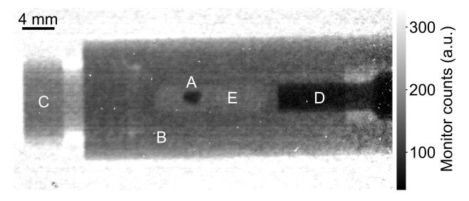
Figure 3: Conventional, flat-field normalized neutron radiography of the clamp cell used to pressurize the  $HgCr_2Se_4$  sample (A). The cell body (B) and the locking nut (C) are made of hardened copper-beryllium. A tungsten-carbide piston (D) is pressed into the sample space (E) filled with a liquid pressure medium.
