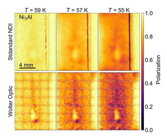
Figure 4: Neutron polarization images of a Ni<sub>3</sub>Al sample at 59 K, 57 K and 55 K. The top row are images obtained with standard neutron depolarization imaging. The bottom row images are the result of stitching 35 images obtained with the polarized neutron microscope. The dashed square delimits the sample edges.
