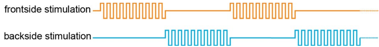
Figure 9 | Illustration of a long-duration current waveform using double-side electrode stimulation for reduced muscle fatigue. The frontside and backside electrode sites are controlled to alternatively deliver the stimulation current.
