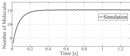
Fig. 3. The time-varying expected number of molecules observed  $\bar{N}_{\text{agg}}^\dagger(\vec{x}_i, t|\lambda)$  versus time  $t$  for  $R_1 = 20 \mu\text{m}$ ,  $\lambda = 7.9 \times 10^{-2}/\mu\text{m}^2$ , and  $\vec{x}_i = (10, 10)$ . For other simulation details, please see Sec. V.
