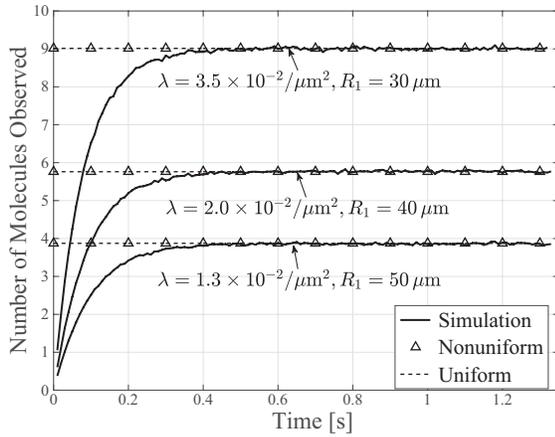
Fig. 5. The expected number of molecules observed at the RX  $\mathbb{E}\{\overline{N}_{\text{agg}}(\vec{b}, t|\lambda)\}$  due to continuous emission at randomly-distributed TXs for different environmental radius  $R_1$ . The average number of TXs is 100 and the RX's location is  $(10 \mu\text{m}, 10 \mu\text{m})$ .
