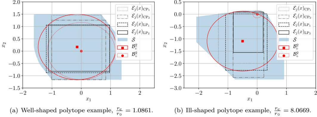
FIGURE 1. Comparison of the CP and LP approaches to construct  $\mathcal{E}_j(x) \subseteq \bar{\mathcal{S}}$ . (a)  $\bar{\mathcal{S}}$  is distributed in a fairly uniform manner around the origin. All the approaches provide close behaviors. (b)  $\bar{\mathcal{S}}$  is distributed in a relatively uneven manner around the origin. The approaches  $\text{CP}_2$  and  $\text{LP}_2$  promote more symmetric constructions compared to the approaches  $\text{CP}_1$  and  $\text{LP}_1$ .
