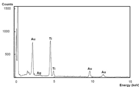
**Figure 6:** Elemental analysis of 0.5 (wt.%) Ag/TiO<sub>2</sub> nanocomposite
