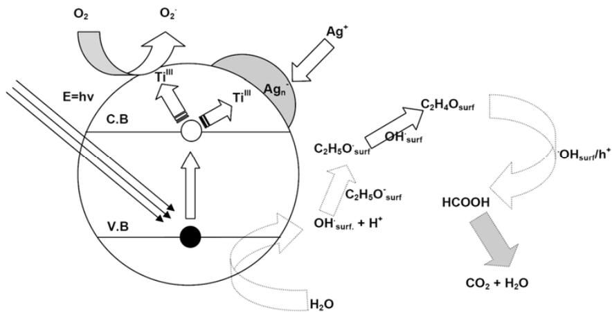
**Figure 2:** Proposed mechanism for the photoreduction of Ag onto TiO<sub>2</sub> in ethanol-water media
