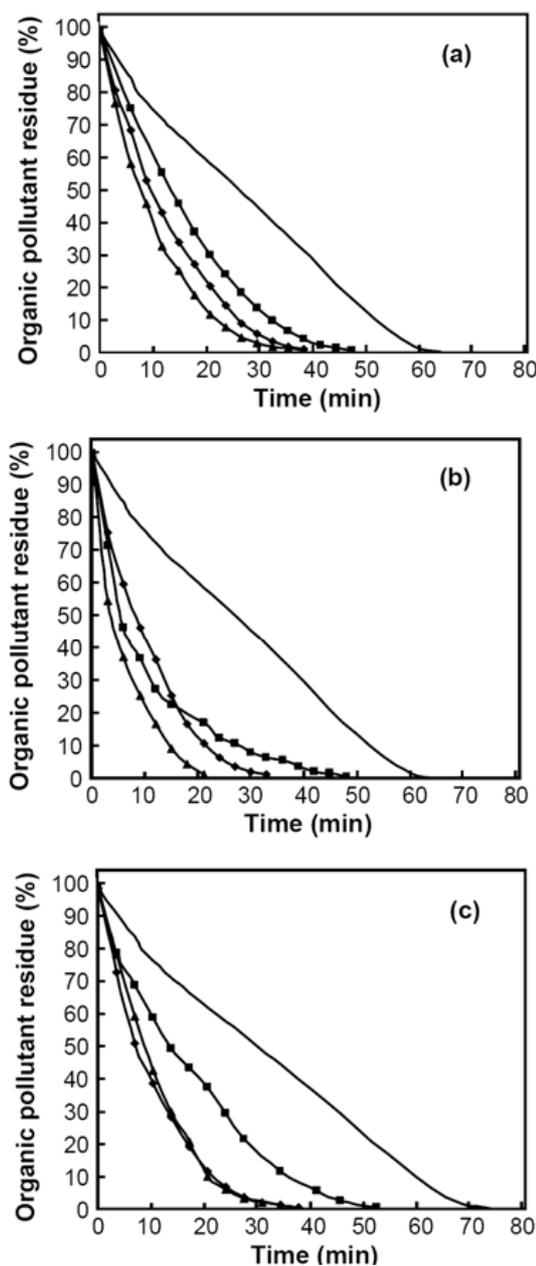
**Figure 7:** Photocatalytic activity of  $\text{TiO}_2$  and  $\text{Ag}/\text{TiO}_2$  nanocomposites: ( $\blacktriangle$ ) 0.05 wt.%  $\text{Ag}/\text{TiO}_2$ , ( $\blacksquare$ ) 0.1 wt.%  $\text{Ag}/\text{TiO}_2$ , ( $\blacklozenge$ ) 0.5 wt.%  $\text{Ag}/\text{TiO}_2$ , ( $\times$ ) Non-modified  $\text{TiO}_2$  (P25), (a) non-calcined, (b)  $\text{Ag}/\text{TiO}_2$  300°C and (c)  $\text{Ag}/\text{TiO}_2$  400°C.
