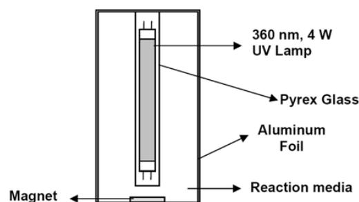
**Figure 1:** Reaction vessel for photocatalytic reduction of Ag on to  $\text{TiO}_2$
