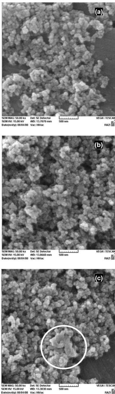
**Figure 5:** SEM images of (a) 0.5% Ag/TiO<sub>2</sub>, (b) 0.5% Ag/TiO<sub>2</sub> 300 °C calcined and (c) 0.5% Ag/TiO<sub>2</sub> 400 °C calcined
