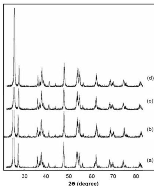
**Figure 4:** XRD patterns of the  $\text{Ag}/\text{TiO}_2$  nanocomposites synthesized using different amounts of doped Ag: (a) 0.05, (b) 0.1 and (c) 0.5 (wt.%)  $\text{Ag}/\text{TiO}_2$  nanocomposites and (d)  $\text{TiO}_2$  (P25)
