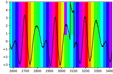
Figure 8: Classifier with  $n_0 = 10$ ,  $n^{n_0} = 10$  applied to wave with pulse anomaly injected at time stamp 3072
