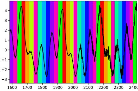
Figure 11: Classifier with  $n_0 = 10$ ,  $n^{n_0} = 8$  applied to wave with slightly increased white noise ( $\sigma = 4.77$ ) starting at time stamp 2048
