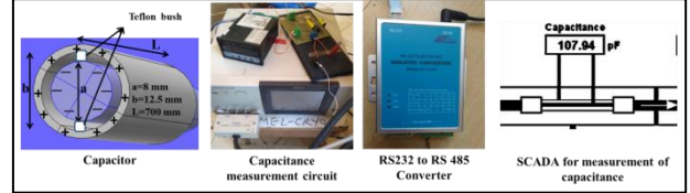
Fig. 3: Capacitance measurement setup
