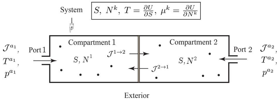
Figure 3.3: Simple open system with a single chemical component experiencing diffusion between two compartments, and transfer into or out of the system through two ports.
