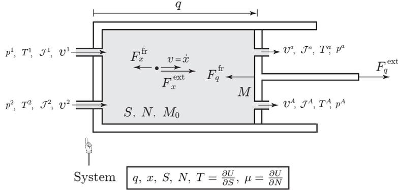
Figure 3.1: Simple open system given by a flowing fluid carrying kinetic energy into a piston device.
