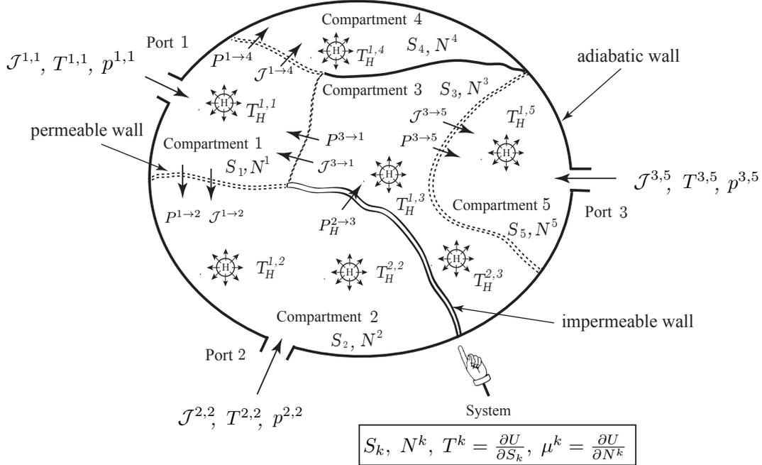
Figure 4.1: Open system with a single species experiencing internal diffusion and heat transfer between several compartments, and transfer into or out of the system through several ports.
