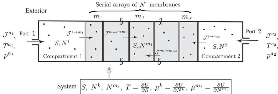
Figure 3.4: Simple open system with diffusion of a single chemical species through a composite membrane made of a serial array of  $N$  elements.
