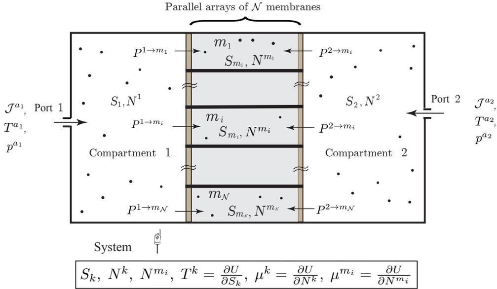
Figure 4.3: Non-simple open system with heat conduction and diffusion of a single chemical species through a composite membrane made of a parallel array of  $\mathcal{N}$  elements.
