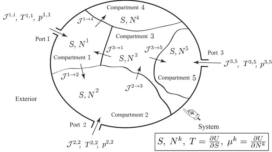
Figure 3.2: Simple open system with a single species experiencing internal diffusion between several compartments, and transfer into or out of the system through several ports.
