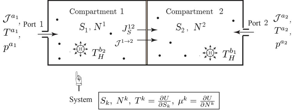
Figure 4.2: Non-simple open system with a single chemical component, experiencing diffusion and heat conduction between two compartments, and transfer into or out of the system through two ports.
