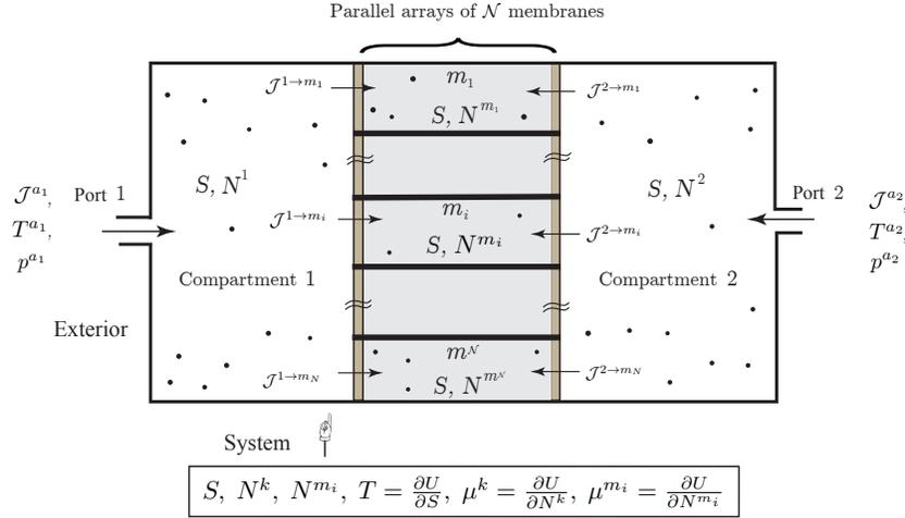
Figure 3.5: Simple open system with diffusion of a single chemical species through a composite membrane made of a parallel array of  $\mathcal{N}$  elements.
