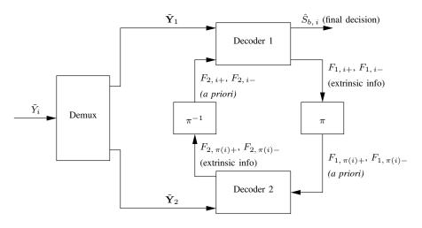
Figure 2. Turbo decoder.
