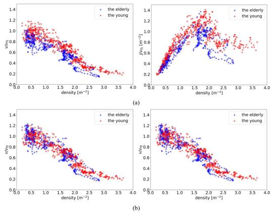
Fig.8. Normalized fundamental diagrams based on the free velocities obtained in two different ways, (a) directly measured free velocity from individual movement, (b) the mean velocity for pedestrian movement under low densities.
