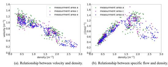
Fig.4. Fundamental diagrams obtained from three different measurement areas.
