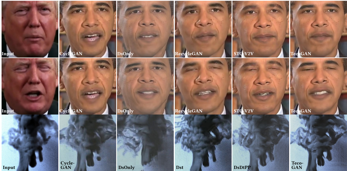
Fig. 8. When learning a mapping between Trump and Obama, the CycleGAN model gives good spatial features but collapses to essentially static outputs of Obama. It manages to transfer facial expressions back to Trump using tiny differences encoded in its Obama outputs, without understanding the cycle-consistency between the two domains. Being able to establish the correct temporal cycle-consistency between domains, ours, RecycleGAN and STC-V2V can generate correct blinking motions, shown in Sec. 4.7 of the supplemental web-page. Our model outperforms the latter two in terms of coherent detail that is generated. Obama and Trump video courtesy of the White House (public domain).
