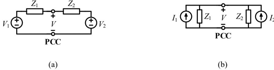
Fig. 1 An interconnected system. (a) Thevenin's equivalence; (b) Norton's equivalence.
