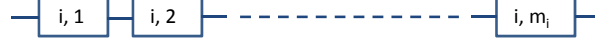
FIG. 2: Failure by the i th path at time t requires m_i independent failures to occur in any order, with the last failure at time t (Eq. 5).
