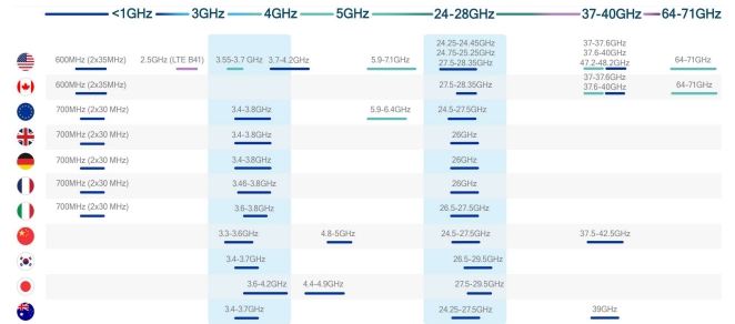
FIGURE 3. Global snapshot of 5G spectrum (blue: Licensed, green: unlicensed/shared, purple: existing bands) [7].
