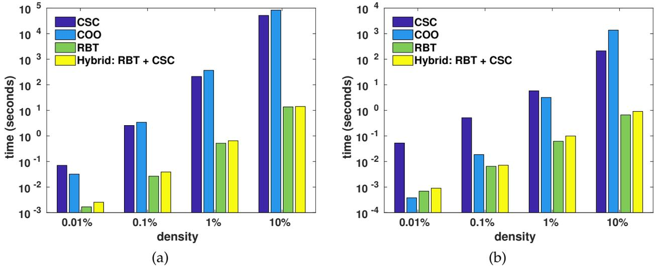
**Figure 6:** Wall-clock time taken to insert elements into a  $10,000 \times 10,000$  sparse matrix to achieve various densities of non-zero elements. In (a), the elements are inserted at random locations in random order. In (b), the elements are inserted in a quasi-ordered fashion, where each new inserted element is at a random location that is past the previously inserted element, using column-major ordering.
