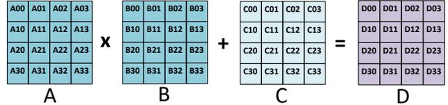
Figure 3: Tensor cores complete one  $4 \times 4$  MACC operation per cycle ( $D = A * B + C$ ). Reproduces Figure 8 in [26].
