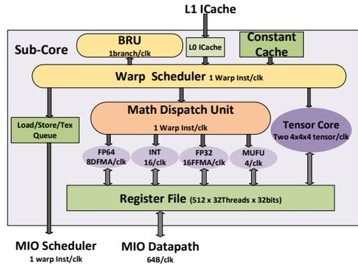
Figure 1: Volta SM Sub-Core (reproduced from [27])
