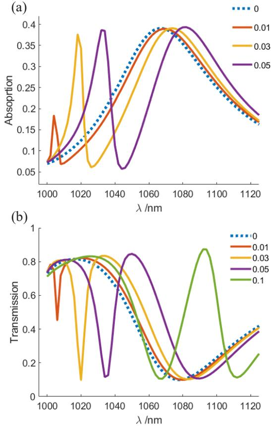
FIG. 3. (Color online) (a) when  $\theta$  is set to  $\pi/4$ , and scan *Ratio*, then a small peak in the absorption spectra grows; (b) the corresponding transmission spectra, and an EIT lineshape appears because of the emergence of a metastable state.
