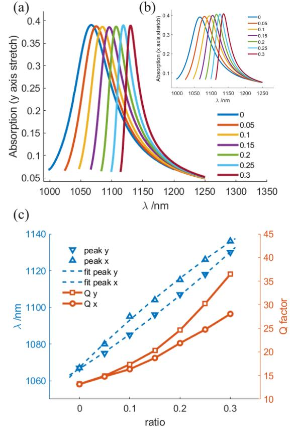
FIG. 2. (Color online) (a) Simulation result of absorption spectra with different *Ratio* in y and (b) x axis on silicon dioxide; (c) wavelength and the Q-factor of *R peak* relative to *Ratio*, and the fitting result of peak to *Ratio* using quadratic function. The fitting residual norm of peak y is 1.0465, for peak x is 2.3805.
