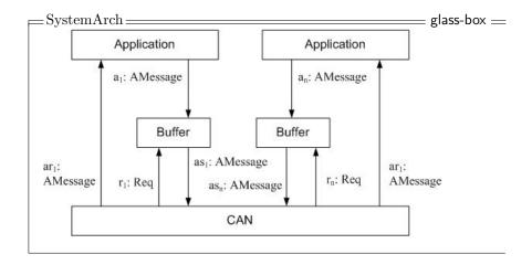
Figure 1: Logical architecture of a CAN-based system
