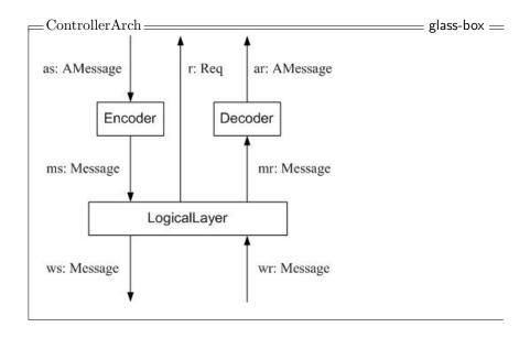
Figure 3: Logical architecture of a Controller component
