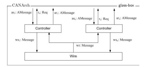
Figure 2: Logical architecture of a CAN component
