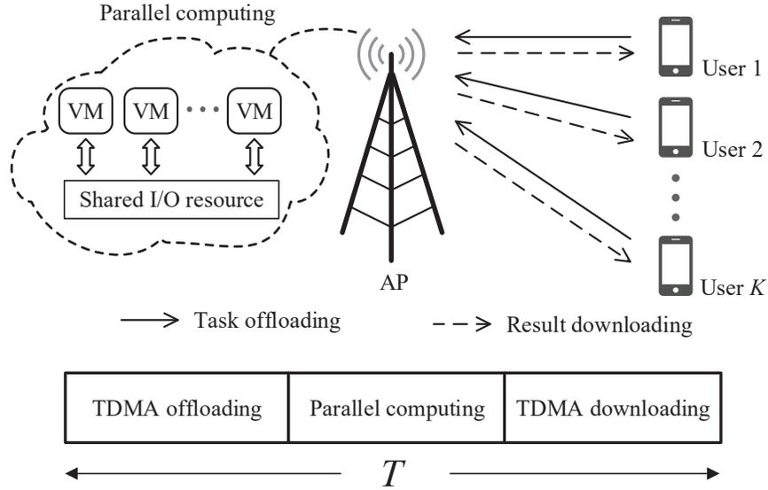
Fig. 1: A multiuser MEC system comprising a single AP and  $K$  users.
