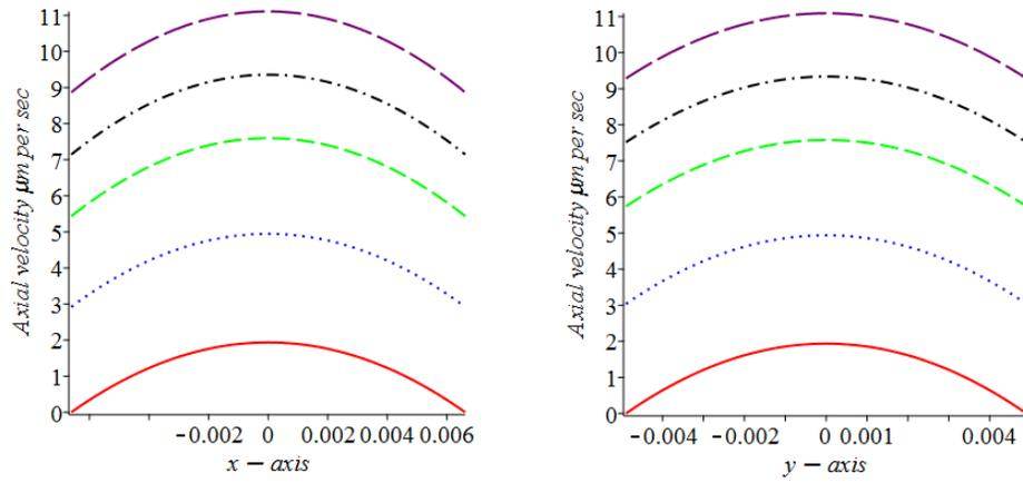
Figure 8: Axial velocity profiles in  $x$  and  $y$  directions obtained from the model having  $a = 6.5 \mu\text{m}$ . and  $b = 4.9 \mu\text{m}$  and various slip lengths  $\ell(\mu\text{m}.)$  of 0.0 (solid line), 6.25(dotted line), 25 (dashed line), 37.5 (dash-dotted line) and 50 (long dashed line).
