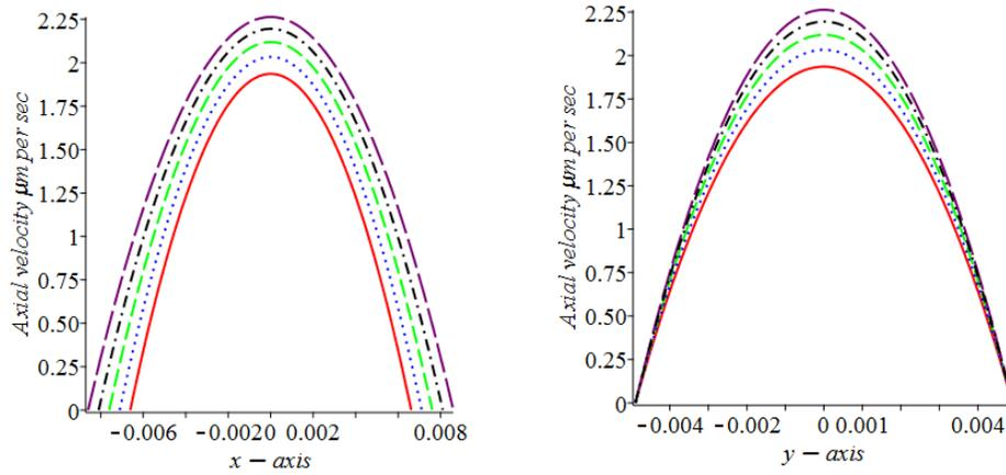
Figure 6: Axial velocity profiles in  $x$  and  $y$  directions obtained from the model with no slip lengths:  $\ell = 0.0$ , and various shapes of cross section.
