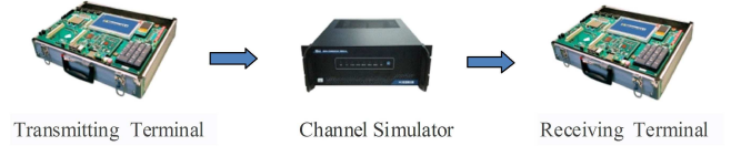
FIG. 6. Chaotic radio wave communication system experimental configuration.
