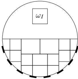
Fig. 6:  $\Omega$  is a disk with diameter of 0.05 and 8 electrodes are covering 47% of the lower half of the boundary. The electrodes are numbered from the left to the right. The resolution partition covers the lower half of the disk. The area  $\omega_I$  allows the presence of bone and blood beside fat.
