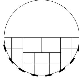
Fig. 5:  $\Omega$  is a disk with diameter of 0.05 and 8 electrodes are covering 47% of the lower half of the boundary. The electrodes are numbered from the left to the right. The resolution partition covers the lower half of the disk.
