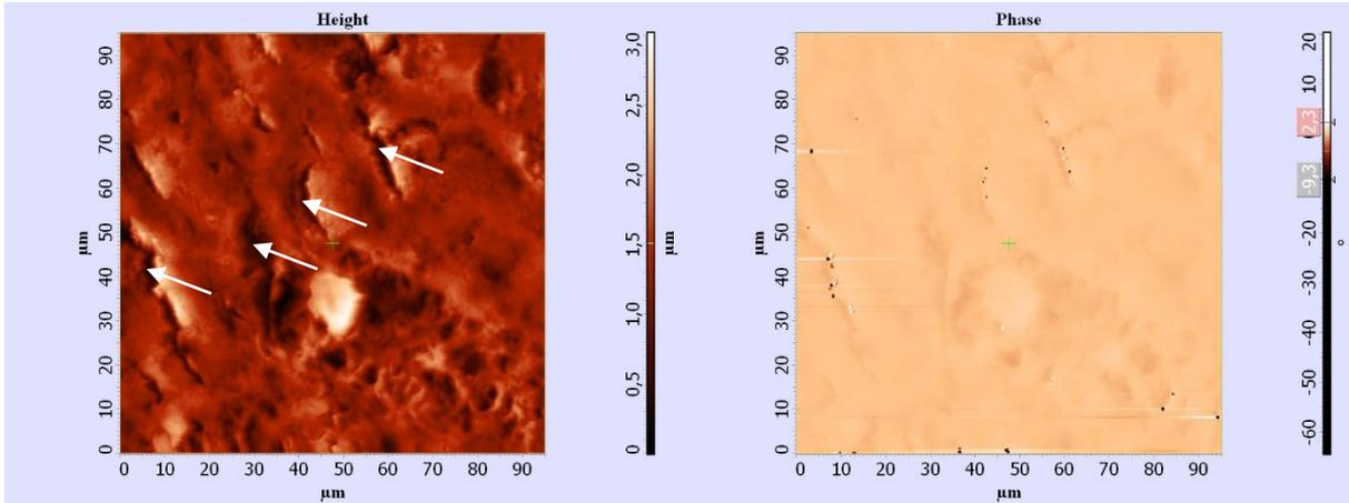
Fig. 4. AFM (left) and MFM (right) images of a sample of the pancreas of the house mouse *Mus musculus*: arrows indicate the capillaries.
