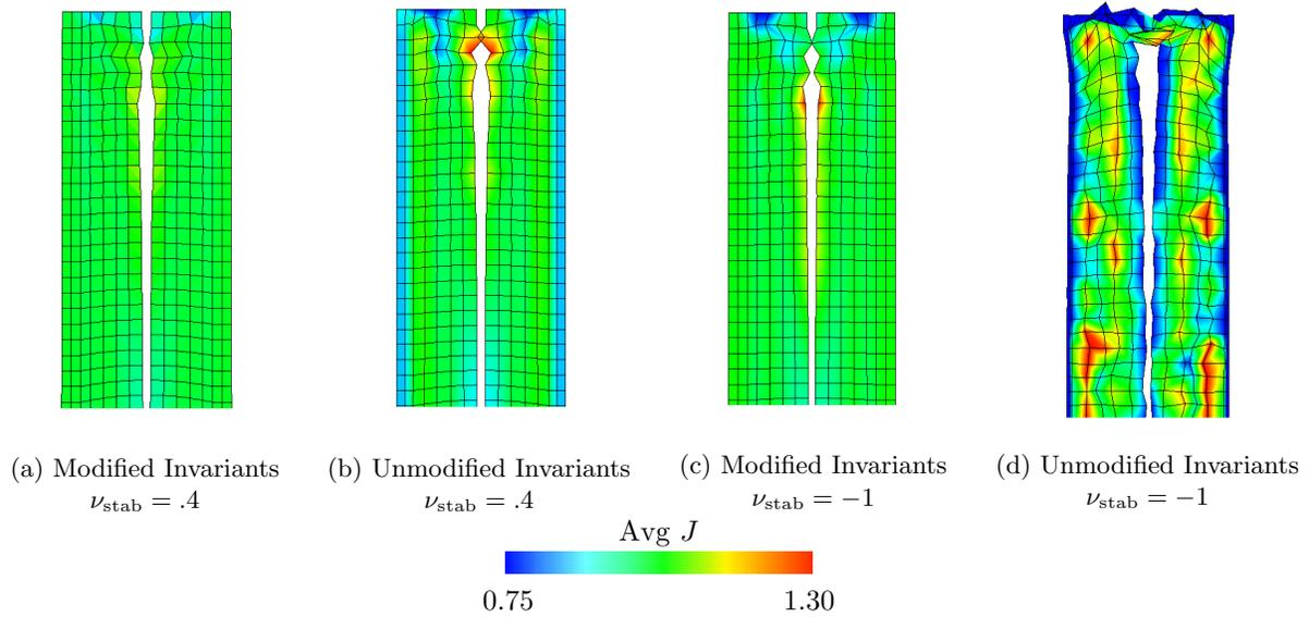
Figure 36: Two dimensional cross-sections of the deformation fields and mean values of  $J$  for the esophageal transport model (Section 5), along with values of  $J$ , at the fixed end of the tube at time  $t = 0.8$  s. Note that panel (d) shows extreme deformations for the case of unmodified invariants and no stabilization.
