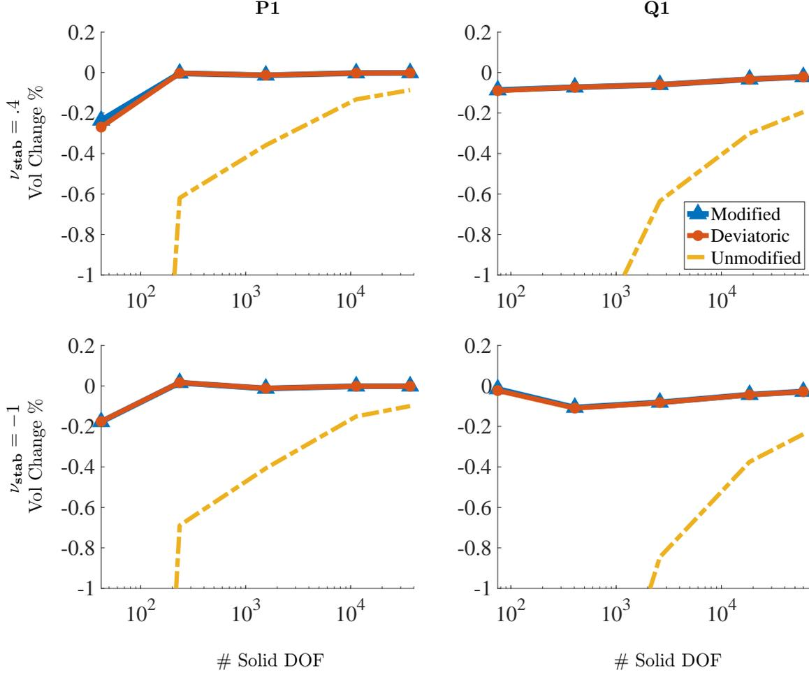
Figure 18: Volume conservation for the anisotropic Cook’s membrane benchmark (Section 4.3) for different choices of elements and numerical Poisson ratio. The DOF range from  $m = 42$  to  $m = 60,025$ , and the  $x$  axis is on a log scale. Omitting the coarsest discretizations ( $m = 42$ ), the largest deviations in total volume among all element types used are approximately .11% for the modified case, 2.2% for the unmodified case, and .11% for the deviatoric case.
