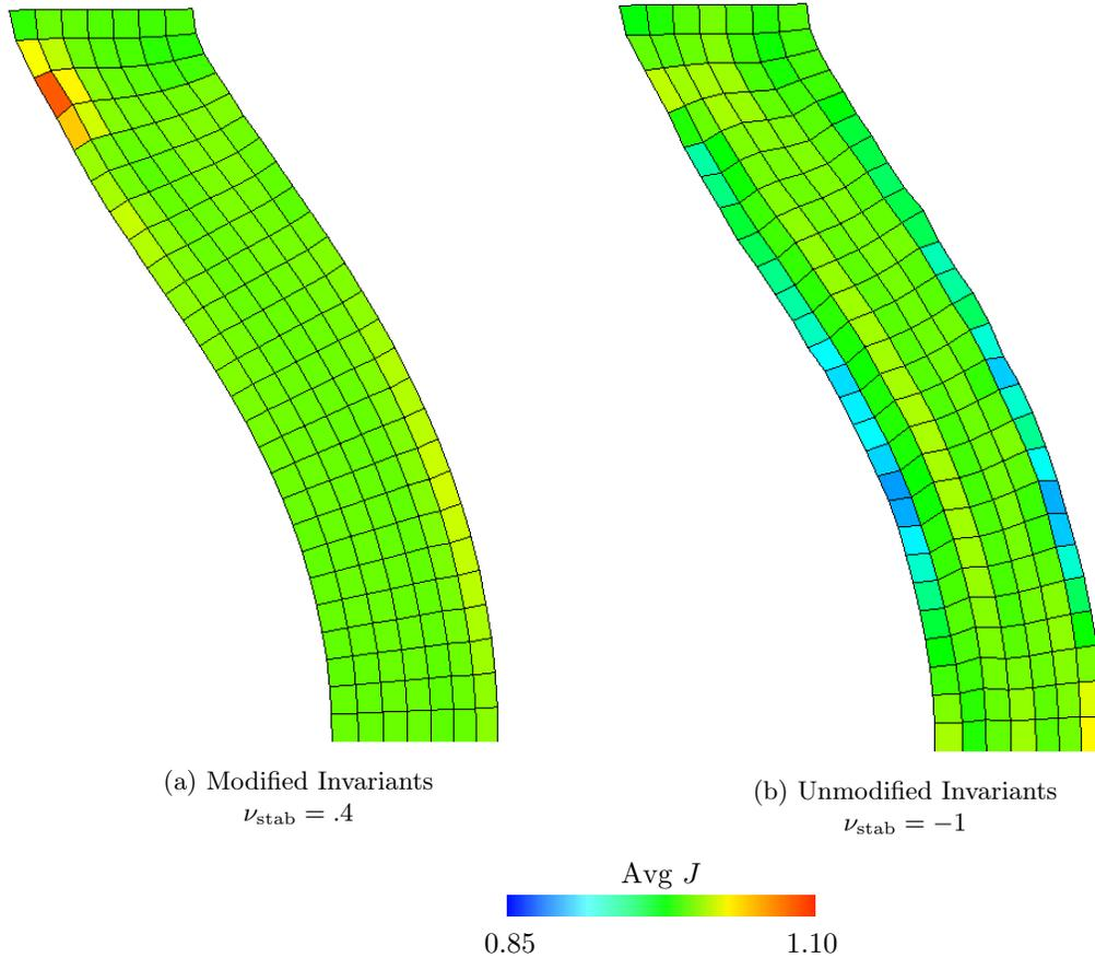
Figure 26: Deformations and mean values of  $J$  of the elastic band (Section 4.5), as also shown in Figure (25). Note the smoother deformations in the panel (a), the modified and stabilized case, as compared to panel (b), the unmodified and unstabilized case.
