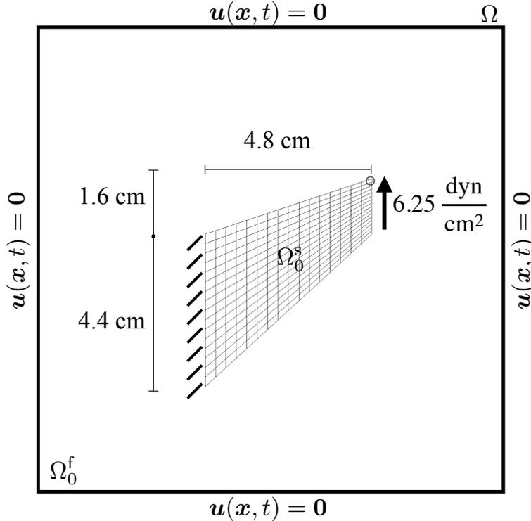
Figure 8: Specifications of the Cook’s membrane benchmark (Section 4.2). The primary quantity of interest is the  $y$ -displacement as measured at the upper right hand corner, indicated by the circle. The structure, shown here in its initial configuration and denoted by  $\Omega_0^s$ , is immersed in a fluid denoted by  $\Omega_0^f$ . The entire computational domain is  $\Omega = \Omega_0^f \cup \Omega_0^s$ . Zero fluid velocity is enforced on the boundary of  $\Omega$ .
