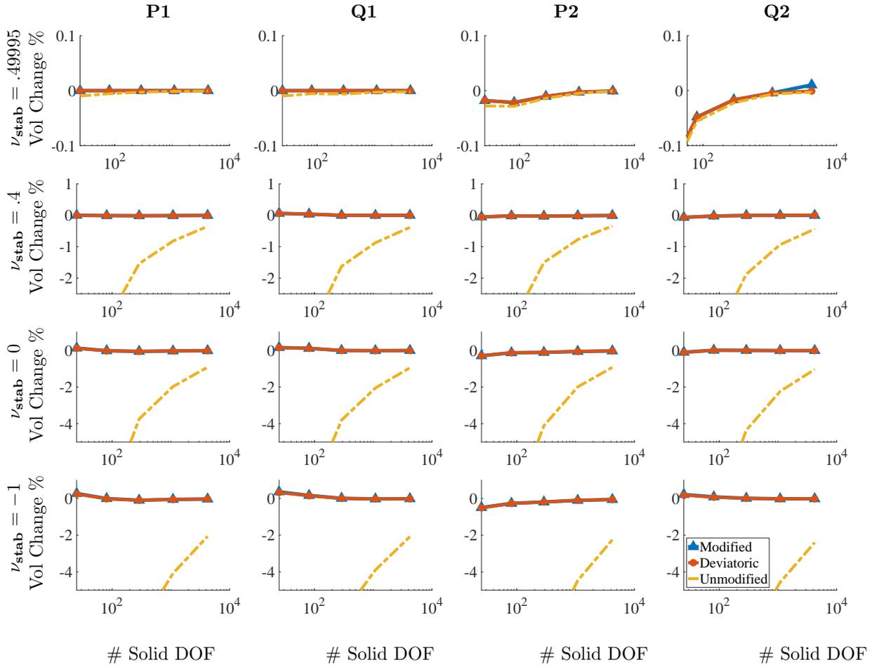
Figure 12: Percent change in total area for different numbers of solid DOF for the Cook’s membrane benchmark (Section 4.2) after deformation. The DOF range from  $m = 25$  to 4225, and the  $x$  axis is on a log scale. Note the different scales on the  $y$ -axes. Omitting the coarsest discretizations ( $m = 25$ ), the largest deviations in total area among all element types used are approximately .10% for the modified case, 7.45% for the unmodified case, and .10% for the deviatoric case.
