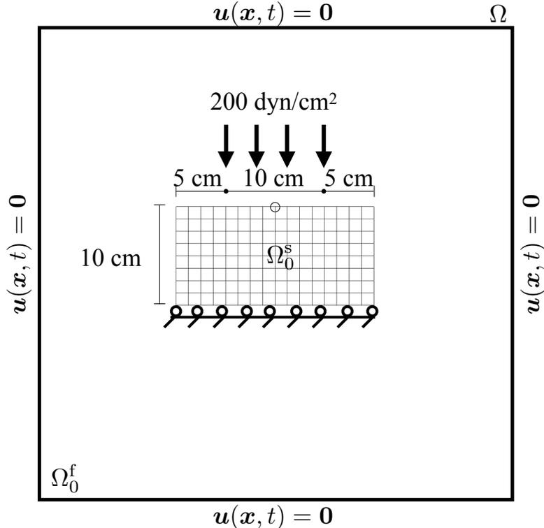
Figure 1: Specifications of the compressed block benchmark (Section 4.1). The quantity of interest is the  $y$ -displacement as measured at the encircled point. The structure, shown here in its initial configuration and denoted by  $\Omega_0^s$ , is immersed in a fluid denoted by  $\Omega_0^f$ . The entire computational domain is  $\Omega = \Omega_0^f \cup \Omega_0^s$ . Zero fluid velocity is enforced on the boundary of  $\Omega$ .
