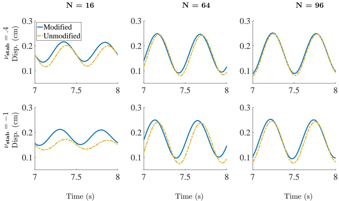
Figure 31: Transient behavior of the elastic band (Section 4.5) for the dynamic version of the test for different discretizations between times  $t = 7.0$  s and  $t = 8.0$  s. Plot shows  $x$ -displacement of point of interest against time.  $N$  describes an  $2N$  by  $N$  Eulerian grid.  $N = 16$  corresponds to  $m = 135$  solid DOF,  $N = 64$  corresponds to  $m = 1456$  solid DOF, and  $N = 96$  corresponds to  $m = 3255$  solid DOF. Results shown here are for **Q2** elements.
