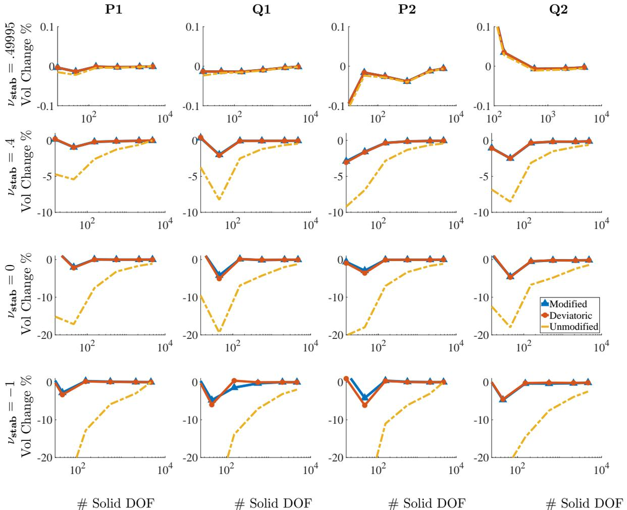
Figure 7: Percent change in total area for different numbers of solid degrees of freedom (DOF) for the compressed block benchmark (Section 4.1) after deformation. The DOF range from  $m = 15$  to 4753, and the  $x$  axis is on a log scale. Omitting the coarsest discretizations ( $m = 15$ ), the largest deviations in total volume among all element types used are approximately 2.1% for the modified case, 14% for the unmodified case, and 2.4% for the deviatoric case.
