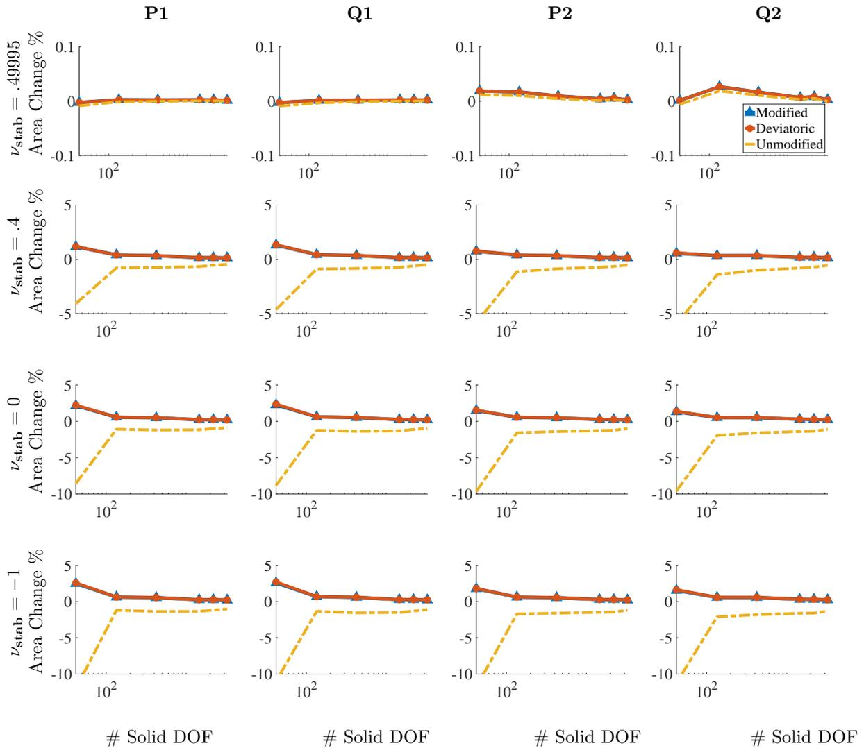
Figure 28: Percent change in total area for different numbers of solid DOF for the steady state elastic band benchmark (Section 4.5) after deformation. The DOF range from  $m = 42$  to 3255, and the  $x$  axis is on a log scale. Omitting the coarsest discretizations ( $m = 42$ ), the largest deviations in total volume among all element types used are approximately 0.69% for the modified case, 2.1% for the unmodified case, and 0.69% for the deviatoric case.
