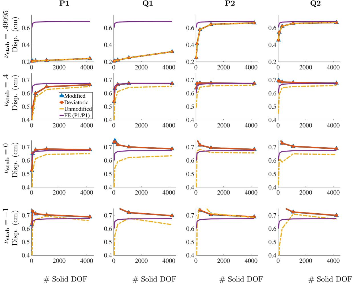
Figure 11: Corner  $y$ -displacement for different number of solid DOF for the Cook's membrane benchmark (Section 4.2) for different choices of elements and numerical Poisson ratios. The solid DOF range from  $m = 25$  to 4225. Notice that each row has the same extents. If a value of  $\nu_{\text{stab}}$  is close to  $\frac{1}{2}$ , low order elements produce volumetric locking, and higher order elements are needed for convergence at reasonable numbers of DOF.
