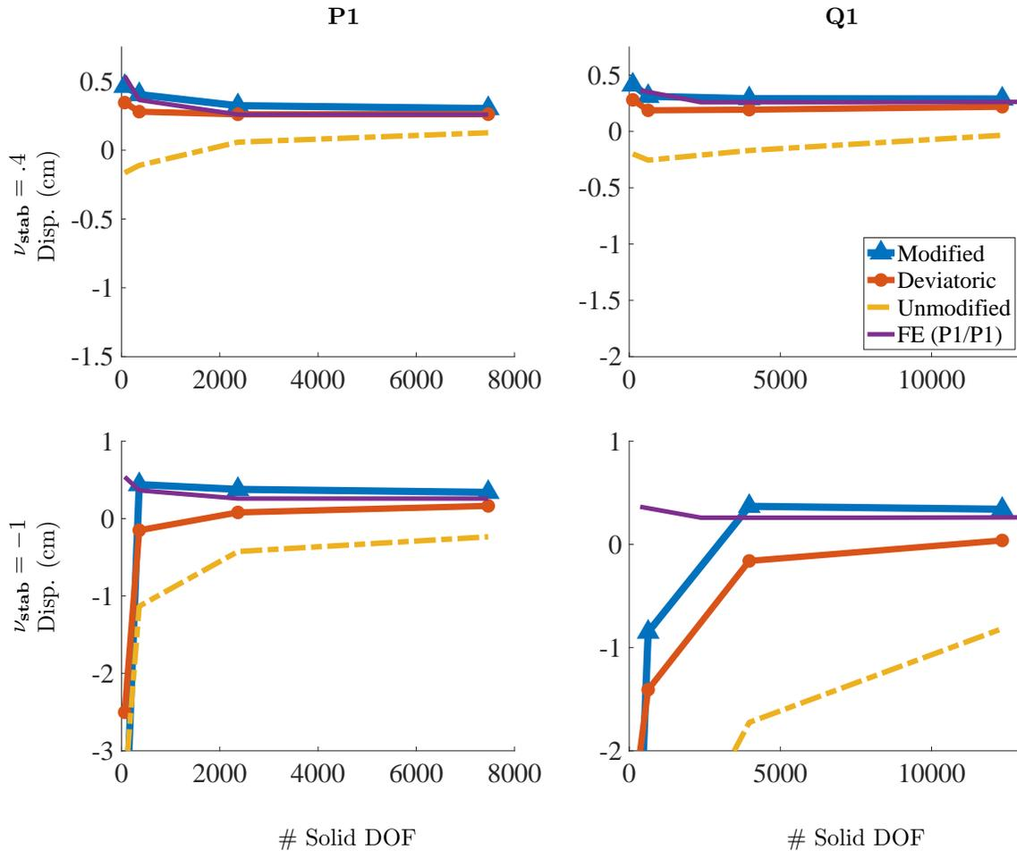
Figure 22: Axial displacement for different solid DOF for the torsion test (Section 4.4) for different choices of elements and numerical Poisson ratio. The solid DOF for the IB tests range from  $m = 65$  to  $m = 12,337$ . Notice that each row has the same  $y$  extents, and each column has the same  $x$  extents. The structural mechanics method is run with an additional discretization of  $m = 17,089$  DOF.
