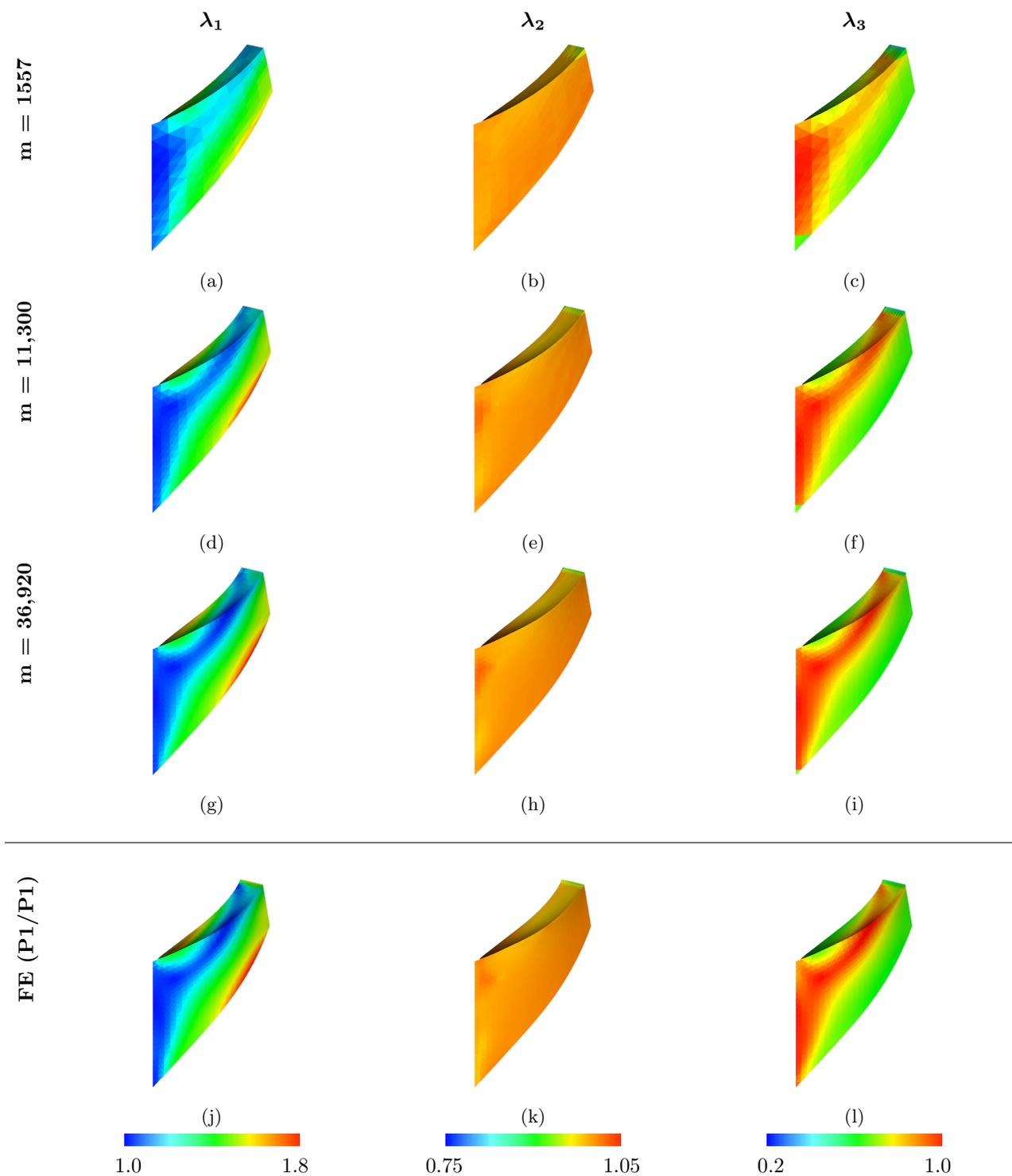
Figure 16: Principal stretches (eigenvalues of  $\mathbb{F}$ ) of the anisotropic Cook's membrane benchmark (Section 4.3) for the IBFE method using  $\mathbf{P1}$  elements with modified invariants and volumetric stabilization ( $\nu_{\text{stab}} = 0.4$ ) and the principal stretches for the FE ( $\mathbf{P1/P1}$ ) method. The solid DOF for the IBFE method are listed in the leftmost column, and the FE ( $\mathbf{P1/P1}$ ) method uses  $m = 36,920$  solid DOF.
