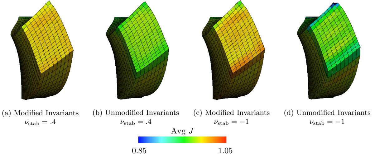
Figure 15: Deformations and mean values of  $J$  of the anisotropic Cook's membrane benchmark (Section 4.3) with zero and finite volumetric energy from a different view; see also Figure (14). The collapsed element in panel (d) is clearly visible.
