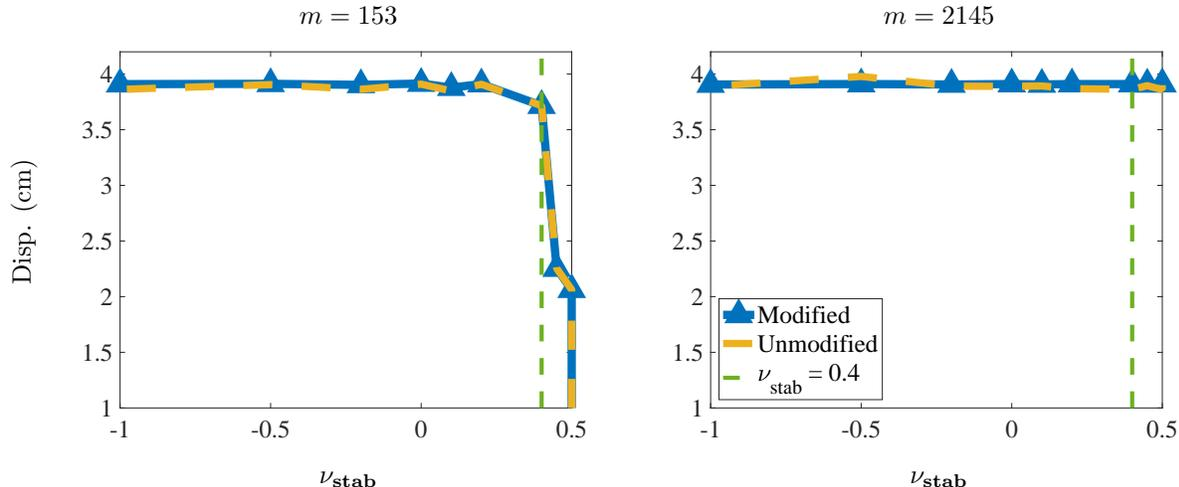
Figure 6: Displacement of the encircled point, shown in Figure (1), plotted against different values of  $\nu_{\text{stab}}$  for the compressed block benchmark (Section 4.1). Results indicate that for a discretization with  $m = 2145$  DOF, the displacement is insensitive to larger values of  $\nu_{\text{stab}}$ . For the coarser case of  $m = 153$  DOF, volumetric locking begins to pollute the solution just past  $\nu_{\text{stab}} = 0.4$ . Results are for **Q1** elements.
