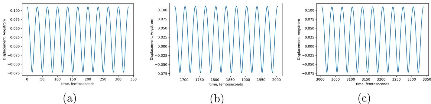
Figure 10: Atomic oscillations, corresponding to mode 2 with amplitude  $0.11 \text{ \AA}$  for three different subintervals: (a)  $0 \dots 10T$ ; (b)  $50T \dots 60T$ ; (c)  $90T \dots 100T$ , where  $T$  is the period of oscillations.
