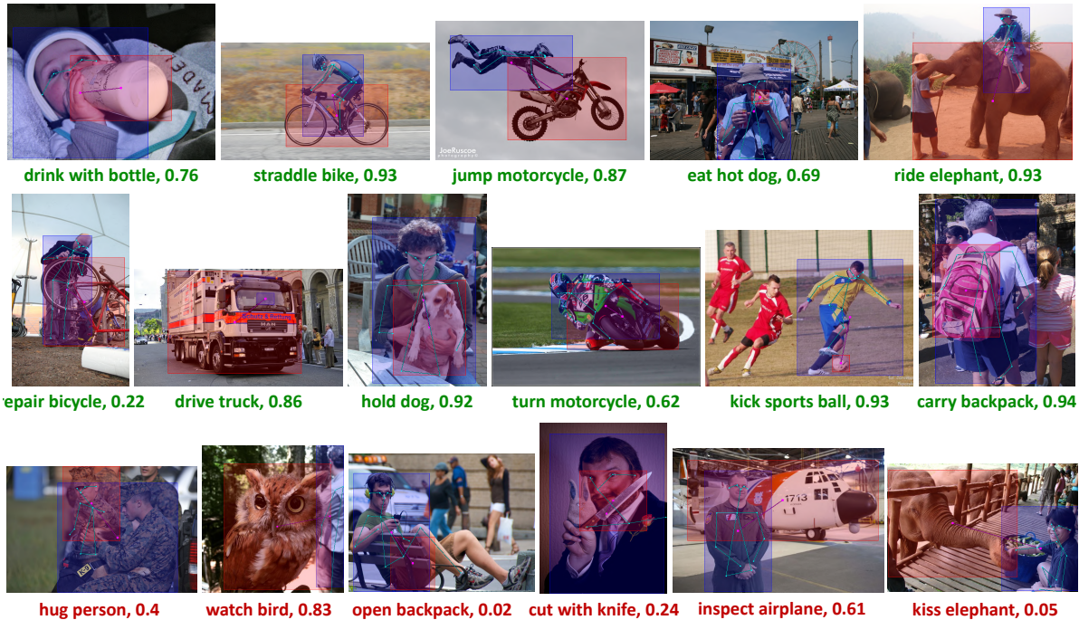
Figure 5: Qualitative results showing top ranking true and false positives for different HOI categories with predicted probability. The blue and red boxes correspond to human and objects detected by a pretrained Faster-RCNN detector respectively. Pose skeleton consists of 18 keypoints predicted by the pretrained OpenPose detector and assigned to the human box.
