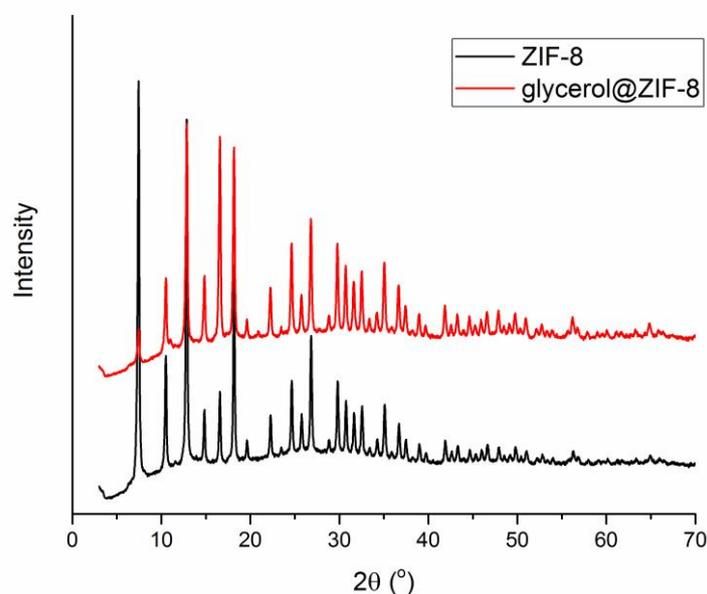
FIG. S1. XRPD patterns of an activated ZIF-8 sample and a glycerol-loaded ZIF-8 sample.
