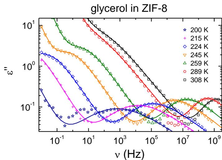
FIG. S6. Frequency dependence of the dielectric loss of glycerol confined in ZIF-8 for different temperatures. The lines through the points are fitted by the sum of two CC functions for the low-frequency effects and a HN function for the main relaxation.
