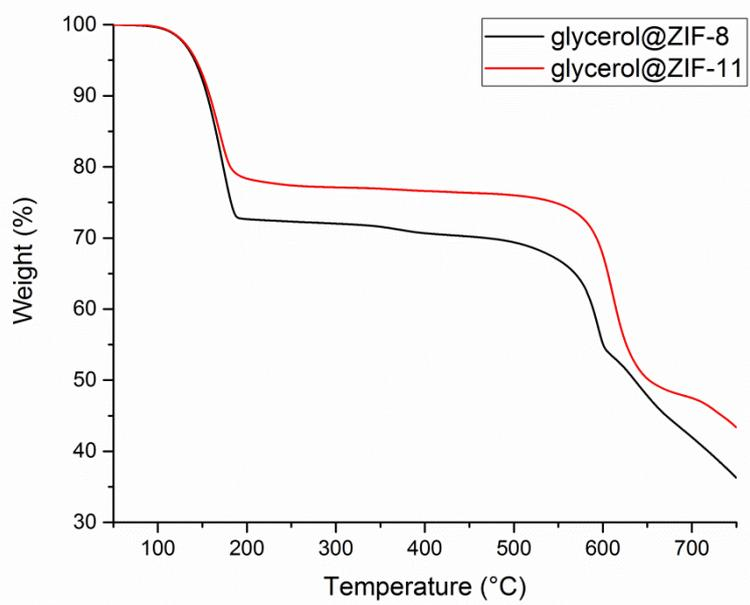
FIG. S3. Overlay of TG curves of ZIFs loaded with glycerol.
