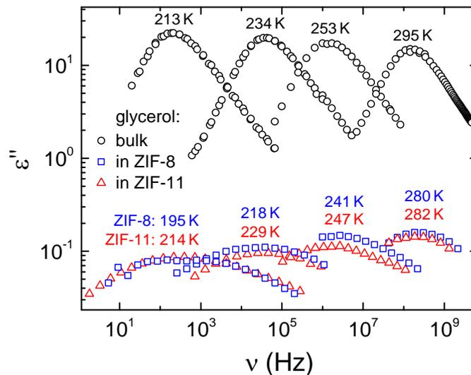
FIG. 3. Frequency dependence of the dielectric loss of glycerol in the  $\alpha$ -peak region (process 1) confined in ZIF-11 (triangles) and ZIF-8 (squares), and of bulk glycerol (circles).<sup>40</sup> The temperatures of the confined systems were selected to achieve an approximate match of the peak frequencies of the bulk results.
