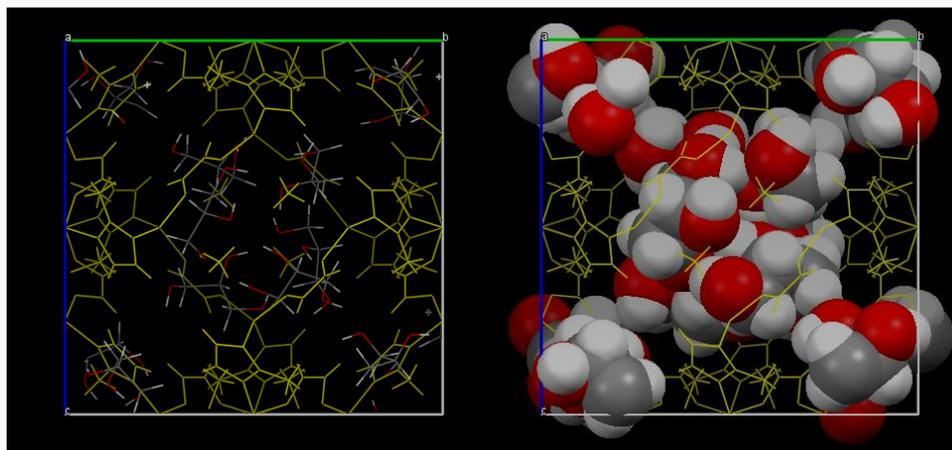
FIG. S4. A representative packing plot of wire model of ZIF-8 (yellow) viewed along the  $a$  axis, in which internal voids are filled with glycerol (12 molecules per unit cell, i.e. 6 molecules per pore).
