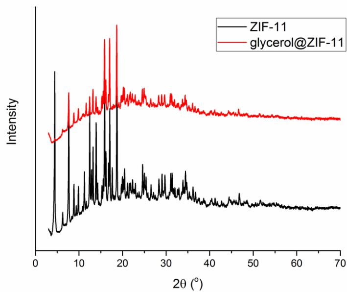
FIG. S2. XRPD patterns of an activated ZIF-11 sample and a glycerol-loaded ZIF-11 sample.
