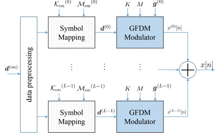
Fig. 3: Core block with multiple prototype pulses.
