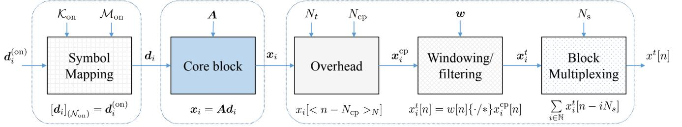
Fig. 1: Multicarrier waveforms generator stages.
