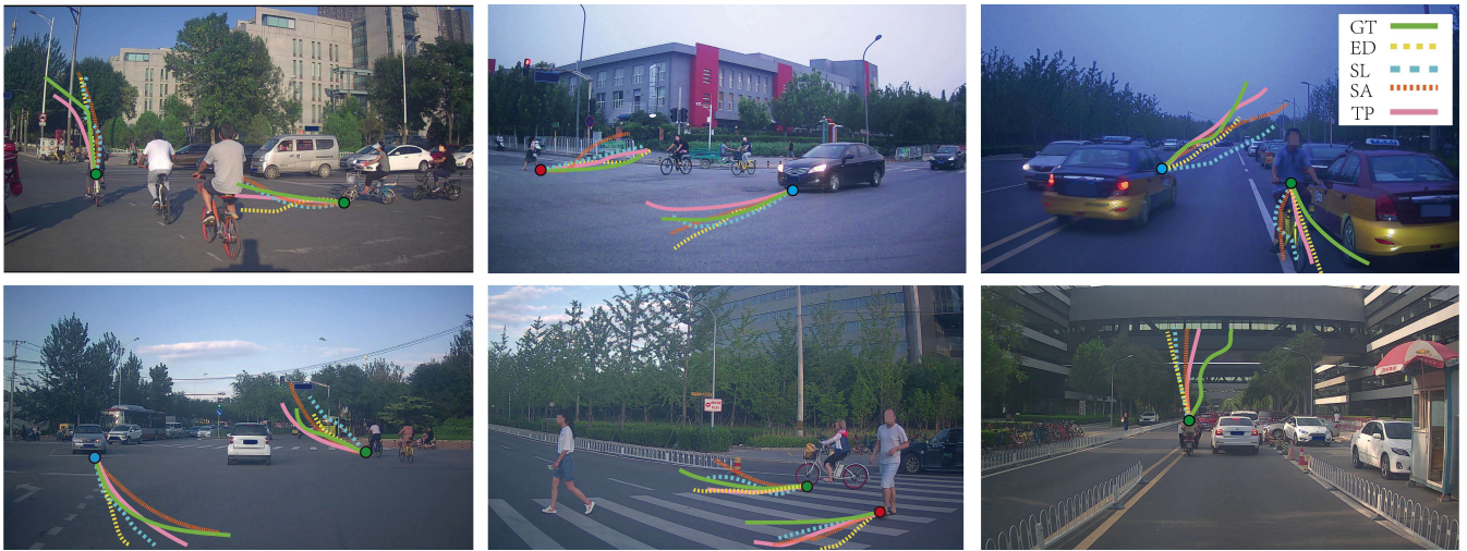
Figure 5: Illustration of our TrafficPredict (TP) method on camera-based images. There are six scenarios with different road conditions and traffic situations. We only show the trajectories of several instances in each scenario. The ground truth (GT) is drawn in green and the prediction results of other methods (ED,SL,SA) are shown with different dashed lines. The prediction trajectories of our TP algorithm (pink lines) are the closest to ground truth in most of the cases.
