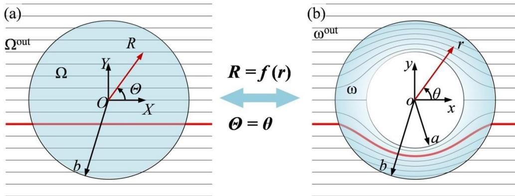
**Fig. 1.** Demonstration of transformation approach for pentamode cloak; (a) Virtual space occupied with homogenous fluid; (b) Physical space with background region  $\omega^{\text{out}}$ , cloak region  $\omega$ ;  $\Omega$  and  $\omega$  have the same outer boundary.
