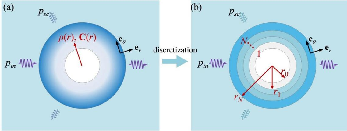
**Fig. 2.** Scattering model of pentamode cloak; (a) A cloak with continuous material parameter is discretized into (b) a cloak with  $N$  layers of orthotropic material.
