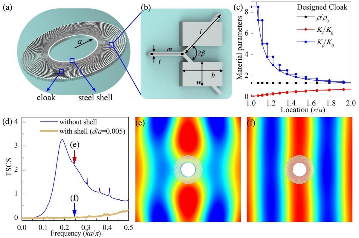
**Fig. 6.** Verification of the proposed boundary scheme through microstructure PM cloak; (a) Microstructure PM cloak with an inner shell; (b) PM unit cell; (c) Material parameter distribution; (d) TSCS for cloak without/with shell; (e)(f) Pressures for cloak without/with shell at  $ka/\pi = 0.25$ .
