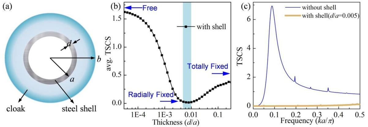
**Fig. 5.** Cloak supported by a traction free inner shell; (a) Schematic configuration; (b) Averaged TSCS with respect to the shell thickness; (c) TSCS for cloak without/with shell.
