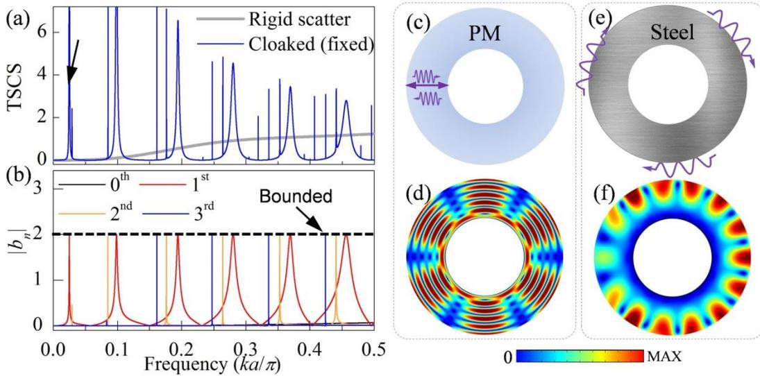
**Fig. 3.** (a) TSCS for a rigid scatter and PM cloak with totally fixed inner surface; (b) Scattering coefficient amplitude corresponding to the first four order; (c) Resonance in the unideal PM cloak is formed by shear wave along the radial direction; (d) Displacement of the PM cloak at resonance. (e) Resonance in ordinary solids is formed by whispering-gallery wave along the circumferential direction; (f) Displacement of a steel shell at resonance.
