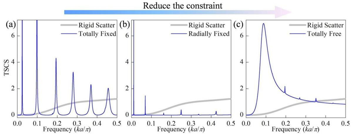
**Fig. 4.** TSCS for a damped cloak (damping ratio 0.5%) with (a) Totally fixed inner surface; (b) Radially fixed inner surface; (c) Free inner surface.
