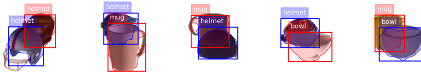
Figure 5: Object segmentation under occlusions. We are able to project the segmented 3D voxels and obtain amodal bounding boxes and segmentation masks, even in the presence of heavy occlusions. We show segmentations specifically from the most heavily occluded camera views.
