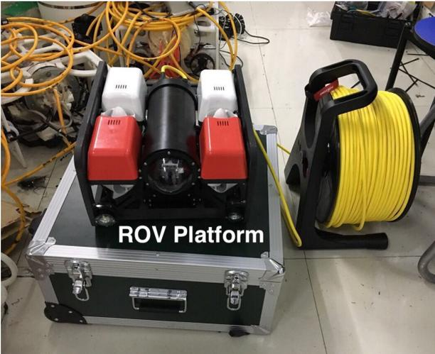
Fig. 8: The designed ROV platform.
