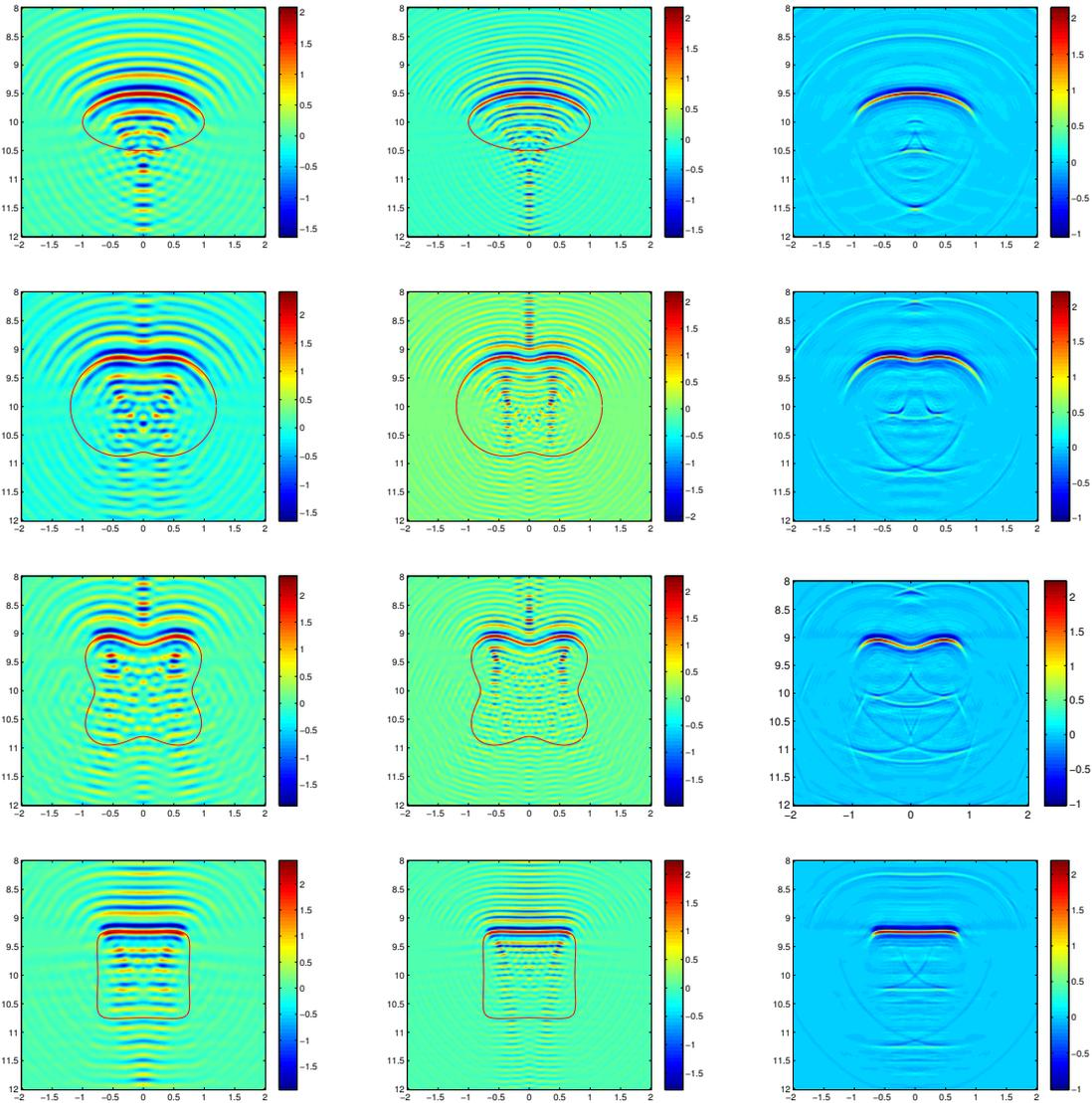
**Figure 3.** Example 2: Imaging results of Dirichlet obstacles with different shapes from top to below. The left column is imaged with single frequency data  $\omega = 3\pi$ , The middle column is imaged with single frequency data  $\omega = 5\pi$  and the right column is imaged with multiple frequency data.
