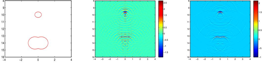
**Figure 5.** Example 3: From left to right, true obstacle model with one circle and one peanut, the imaging result with single frequency data where  $\omega = 3\pi$ , the imaging result with multiple frequency data.
