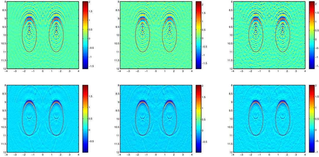
**Figure 6.** Example 4: Imaging results of a Dirichlet obstacle with noise levels  $\mu = 0.2; 0.3; 0.4$  (from left to right). The top row is imaged with single frequency data  $\omega = 4\pi$ , and the bottom row is imaged with multi-frequency data.
