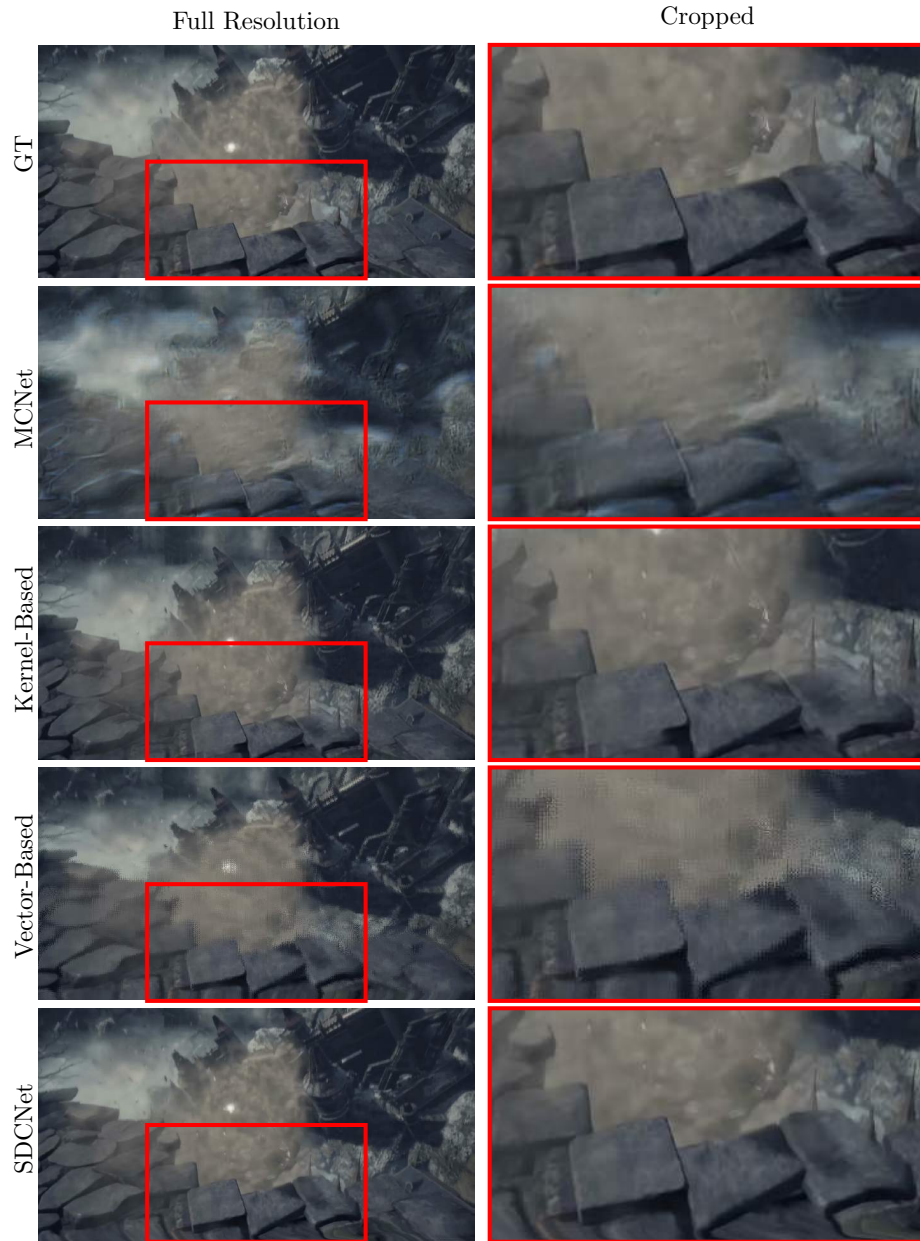
Fig. 7. Comparison of frame prediction for large motion. Expected transformation is an upwards displacement with a slight zoom-in. While the Kernel-based, Vector-based, and SDC-based models were all trained with L1 and fine-tuned with style-loss to promote sharpness, note that the Vector-based result still loses coherence when predicting large displacement. On the other hand, the SDCNet is able to displace as much as the Vector-based model while maintaining sharpness. While the Kernel-based result is relatively sharp, it is conservative about predicting the upwards translation (note the relative distance of tiles to the bottom of the frame compared to the vector and SDC approaches). Further, there is a slight ghosting effect in the right-most tile of the Kernel-based result, which is not present in the SDC result.
