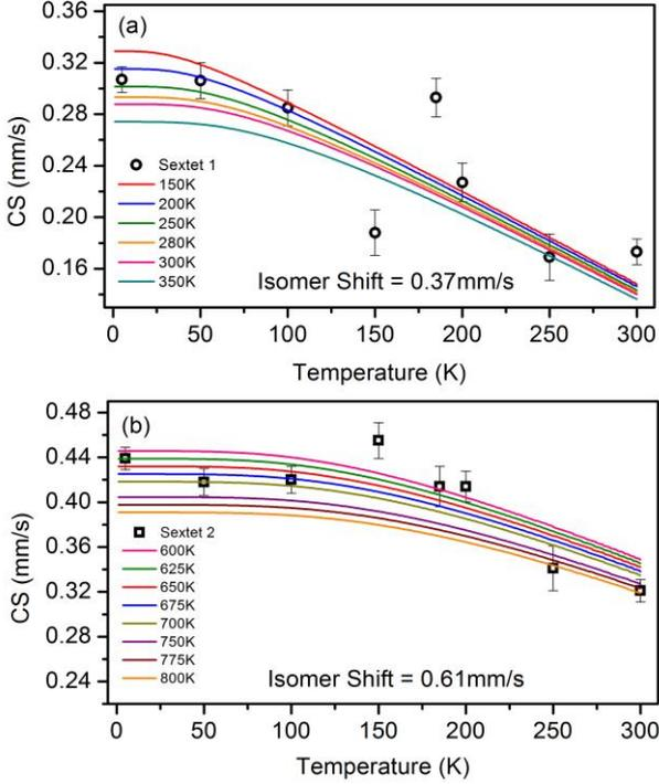
**Figure 7:** Theoretically simulated lines of CSs for given  $\Theta$  (solid lines) and experimental data (points) for Fe<sub>T</sub> (a) and Fe<sub>O</sub> (b).
