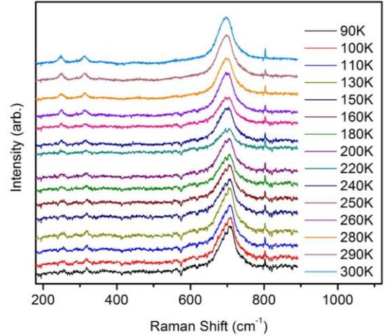
**Figure 8:** Temperature dependence of the Raman Spectrum of Ca<sub>2</sub>FeCoO<sub>5</sub>.
