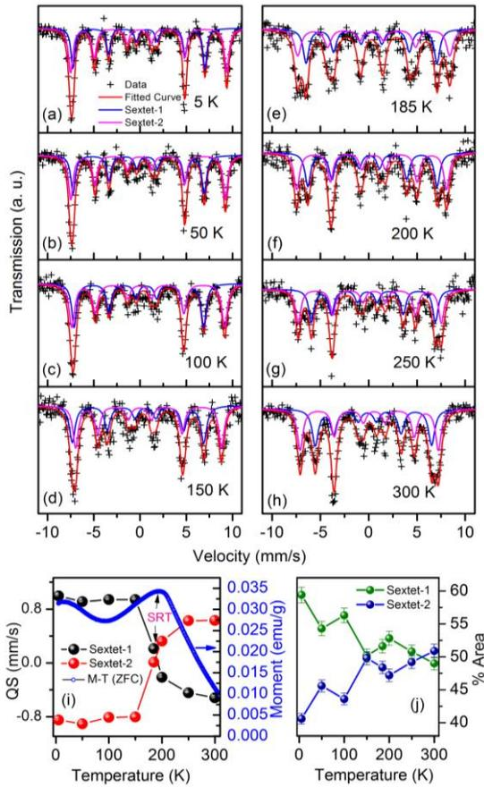
**Figure 4:** Temperature dependent Mossbauer measurements carried out from 300K to 5K (a-h). Panel (i) shows the quadrupole splitting for  $\text{Fe}_T$  and  $\text{Fe}_O$  sites as a function of temperature. ZFC magnetization is also shown to mark the SRT. Panel (j) shown the % area of the overall pattern covered by different sextets representing the Fe occupation at  $\text{Fe}_T$  and  $\text{Fe}_O$  sites.
