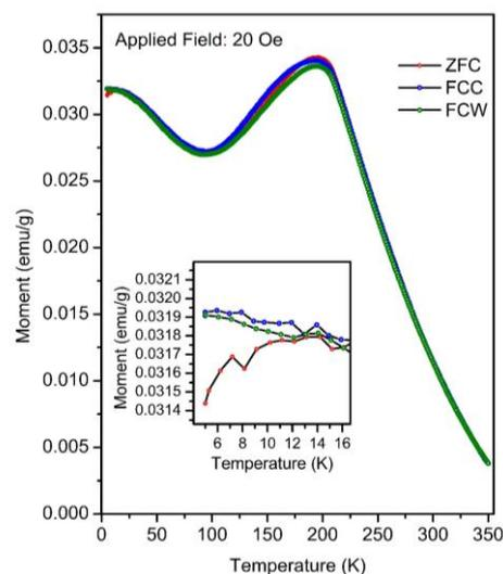
**Figure 3:** Temperature dependent magnetization (M-T) of  $\text{Ca}_2\text{FeCoO}_5$  from 5K to 350K measured in Zero-Field Cooled (ZFC), Field Cooled Cooling (FCC) and Field Cooled Warming (FCW) protocols. The inset shows the zoomed view of low temperature region. The increasing moment below 100K in all the curves also point towards the presence of some degree of spin canting in this system.
