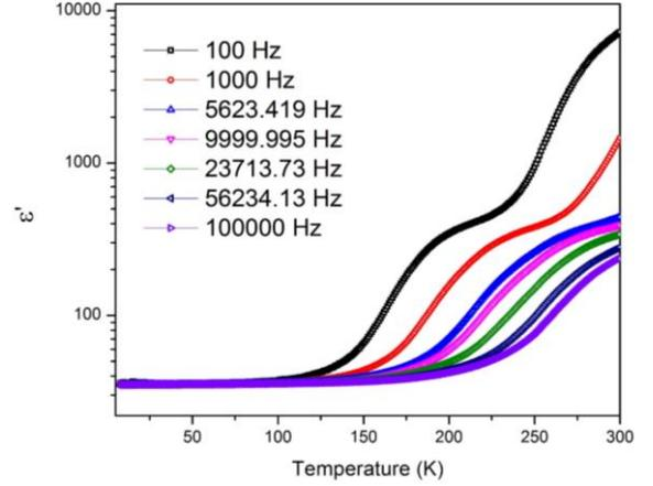
**Figure 10:** The dielectric constant ( $\epsilon'$ ) as a function of temperature for different frequencies showing the presence of frequency dependent relaxations.
