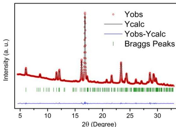
**Figure 1:** Room temperature synchrotron x-ray diffraction pattern of  $\text{Ca}_2\text{FeCoO}_5$  with the Reitveld refinement profile along with the difference pattern and Braggs peaks. The wavelength used was 0.782566 Å, the space group used during refinement was Pbcm,
