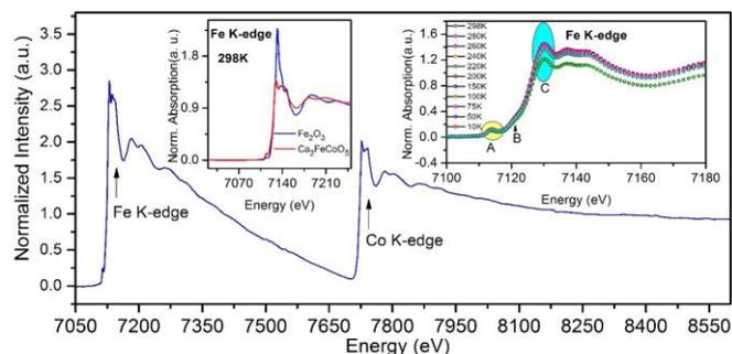
**Figure 2:** XAS data of  $\text{Ca}_2\text{FeCoO}_5$  at Fe and Co K-edge. The first inset shows the Fe k-edge XANES data of  $\text{Ca}_2\text{FeCoO}_5$  along with the reference  $\text{Fe}_2\text{O}_3$  collected at room temperature showing that the oxidation state of Fe in the sample is +3. The second inset shows the temperatures variation of the Fe K-edge XANES indicating that the valence of the cation remains unchanged as the temperature is varied.
