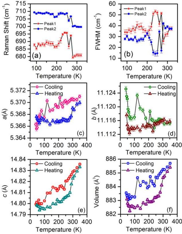
**Figure 9:** The Raman Shift (a) and FWHM (b) of the most prominent modes as a function of temperature and the lattice parameters (c), (d), (e) as a function of temperature obtained from the refinement of SXPD data of  $\text{Co}_2\text{FeCoO}_5$  collected in cooling and heating cycle. The unit cell volume is shown in panel (f).
