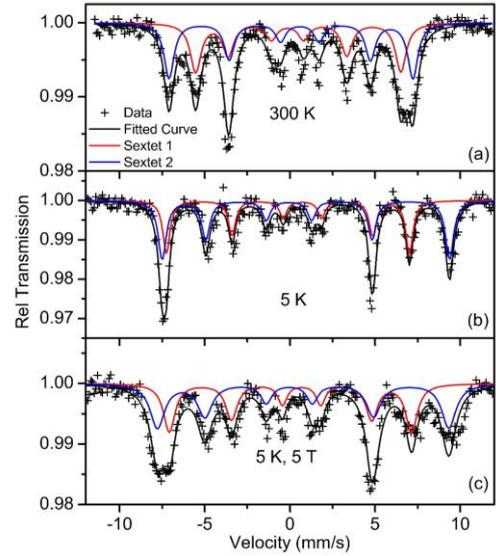
**Figure 5:** Mossbauer spectroscopy data collected at 300 K (a), collected at 5 K (b) and at 5 K under the application of 5 Tesla magnetic field (c) along with the fitting considering the spectrum to be a convolution of two broad sextets representing differently coordinated sub-lattices, namely octahedral and tetrahedral.
