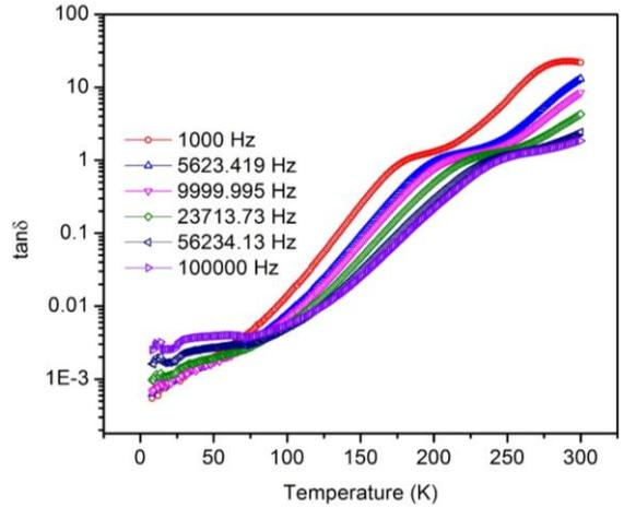
**Figure 11:** The loss tangent ( $\tan\delta$ ) as a function of temperature for different frequencies. The presence of two relaxations is very clear from the figure. The relaxation peaks also show a frequency dependence.
