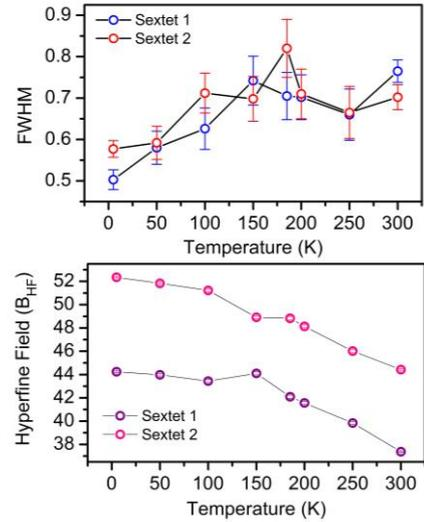
**Figure 6:** The FWHM (a), Isomer Shift (b) and Hyperfine field (c) as a function of temperature. These parameters are obtained by deconvoluting the  $^{57}\text{Fe}$  Mossbauer spectra of  $\text{Ca}_2\text{FeCoO}_5$  collected at different temperatures. The spectra were fitted using two broad sextets representing octahedral and tetrahedral coordination of Fe in the lattice.
