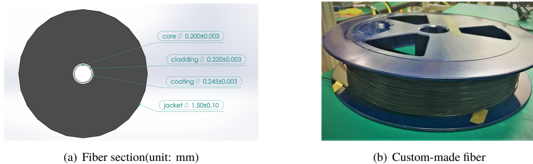
Figure 5. Left figure: cross section of fiber. The core material is high hydroxyl quartz glass, the cladding material is F-doped silica glass, and coating material is bilayer UV-cured acrylic resin. The jacket of the fiber is ETFE. Right figure: the final fiber product.
