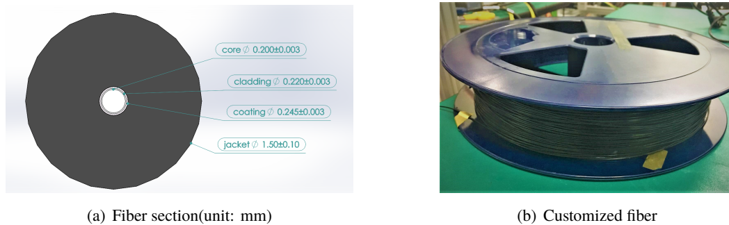
Figure 5. Left figure: cross section of fiber. The core material is high hydroxyl quartz glass, the cladding material is F-doped silica glass, and coating material is bilayer UV curing acrylic resin. The jacket of the fiber is ETFE. Right figure: the final fiber product.
