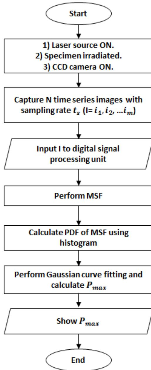
**Fig. 1. Flow diagram for the biospeckle processing algorithm.**
