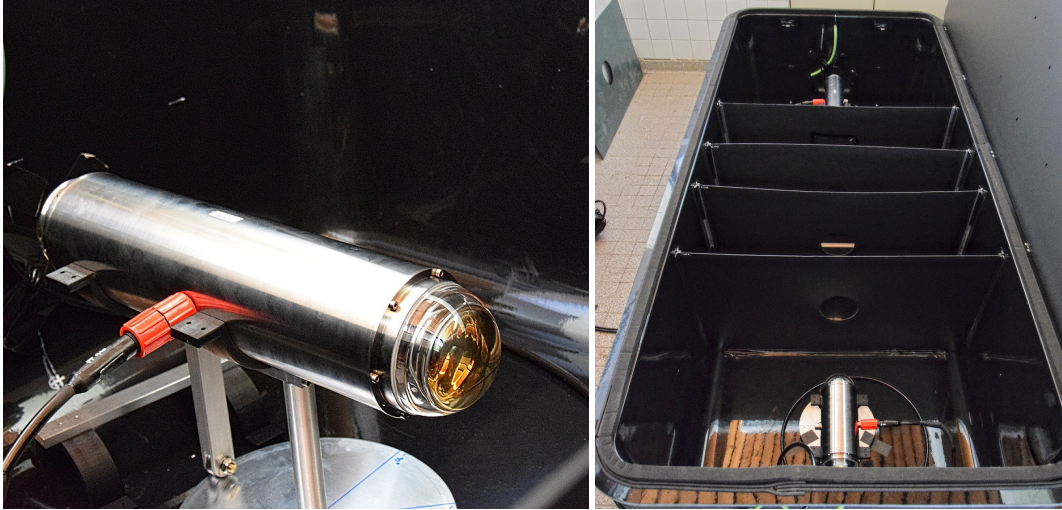
Figure 23: Wet test setup at TUM. The sDOM is fixed to a rotation mount inside a 3\text{ m} \times 1.2\text{ m} pool with baffles for suppressing reflected light. The pool is filled with water during the tests and closed by a light-tight lid.
