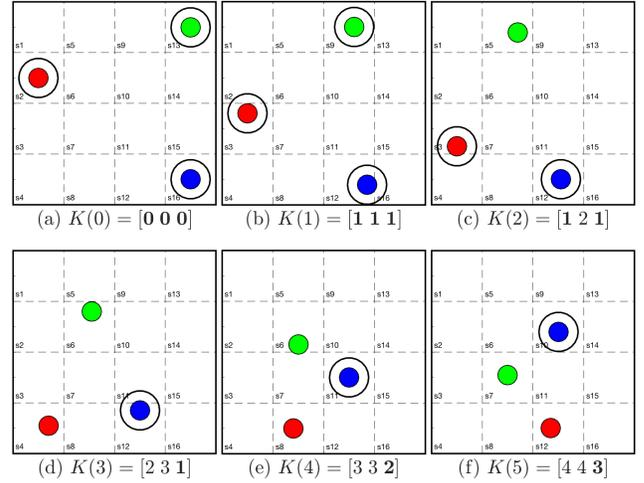
Fig. 1. Frames (a) to (e) correspond to snapshots of a possible asynchronous execution taken at times  $t = 0$  to  $t = 5$ . Robots are enumerated in the order of red, green, blue and local times of robots at each time step are shown below the corresponding frame. Anchoring robots are highlighted with a black circle and the anchor time is shown in bold.
